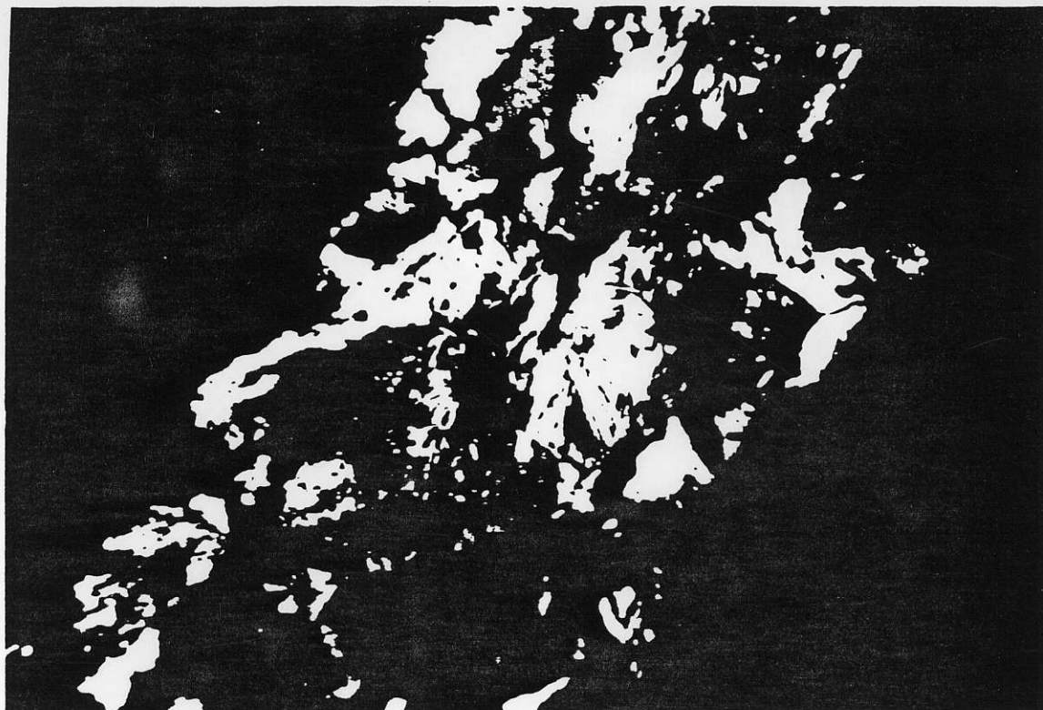
Plate 9-74.9-5. Veinlet of quartz including sheafs of Ba muscovite, Mg chlorite and Mn dolomite.
