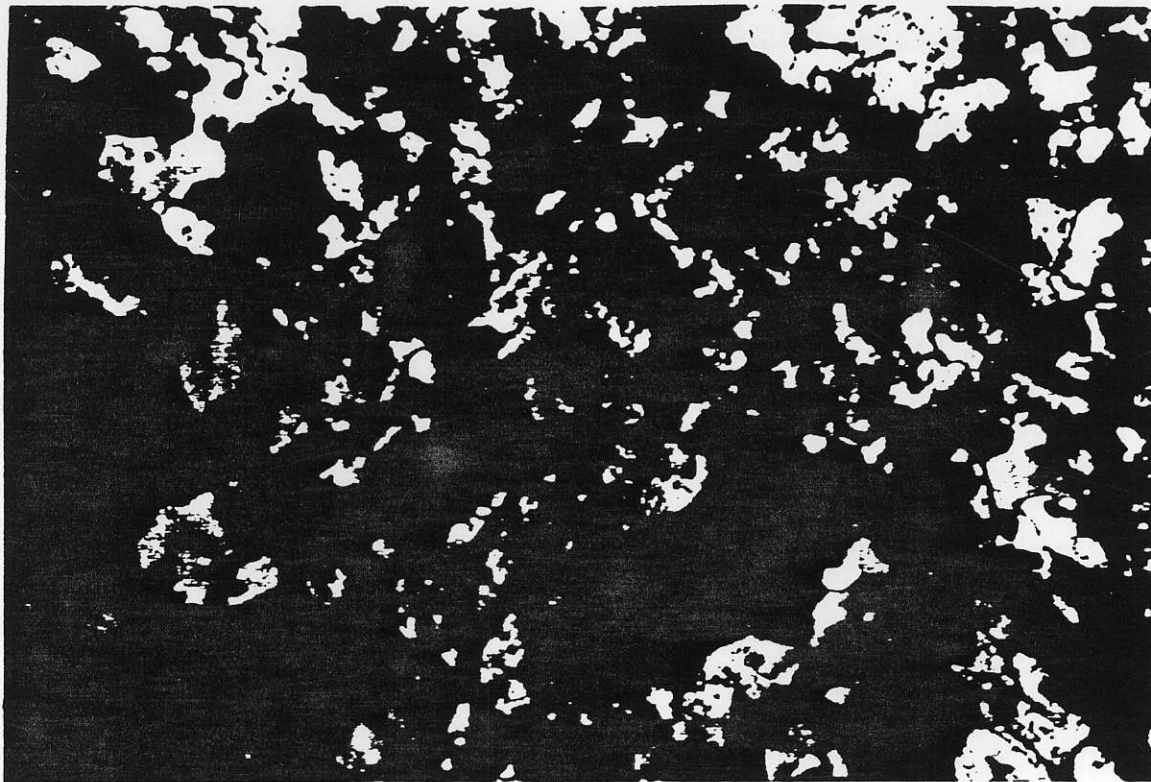
Plate 15-73.0-1. Randomly oriented prismatic quartz with highly variable grain size and sulphide mineral along grain margins.
