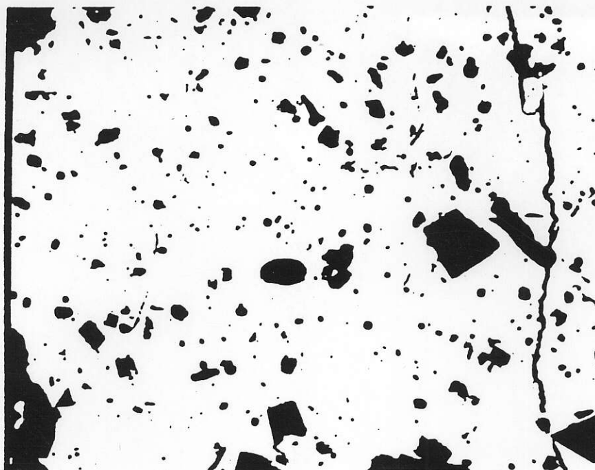
Plate 18-77.0-3. Massive stibnite with included angular pyrite and dolomite, black, and even distribution of \text{PbSbS} , white.
