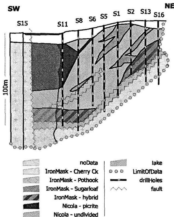
Figure 13. Section 1100 N from Galaxy Copper Ltd. plan showing surface cuts and diamond-drill holes (Preto, 1967, Fig. 14).
