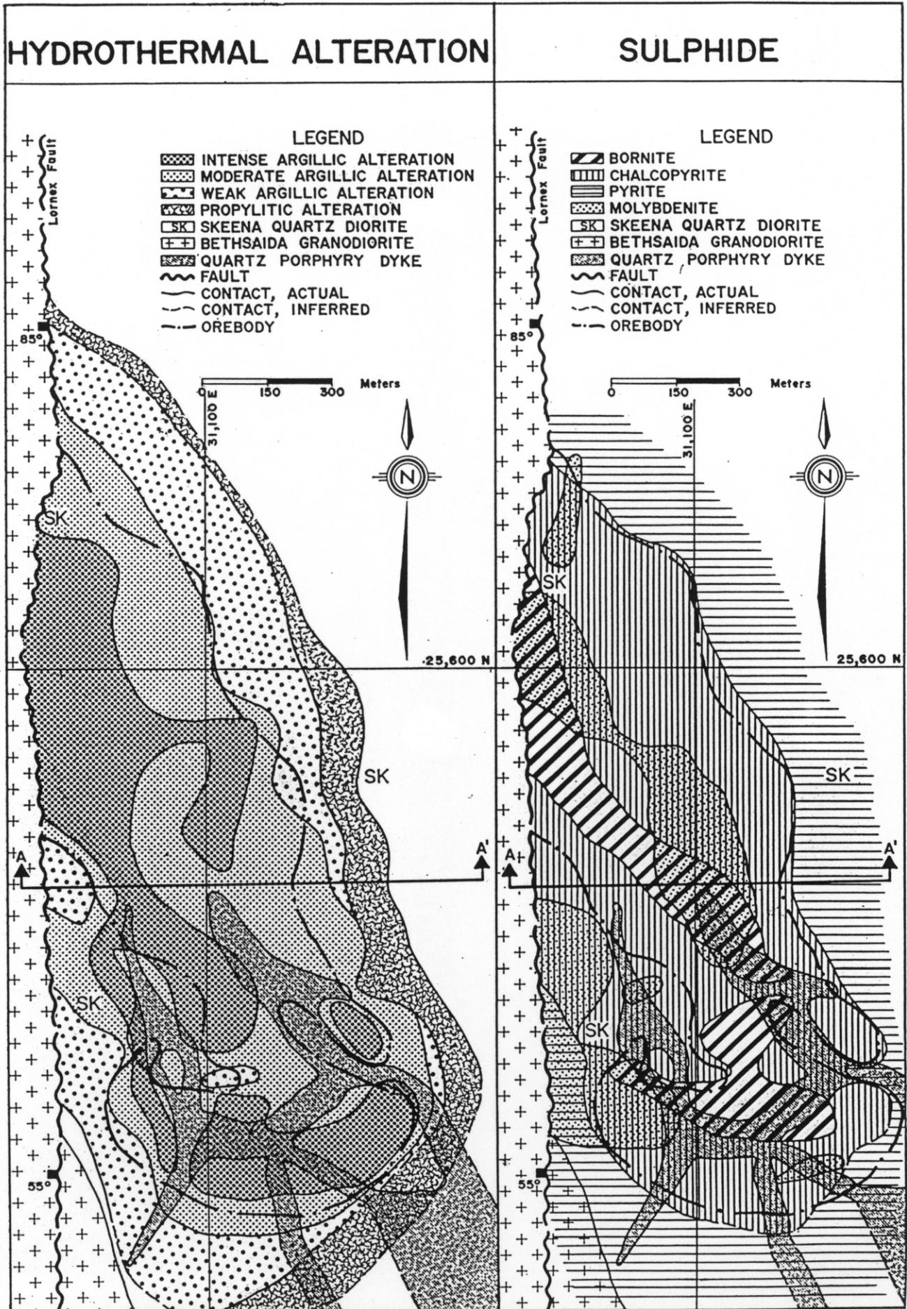
FIGURE 6—Hydrothermal alteration and sulphide mineral zoning at the 1370 level.
