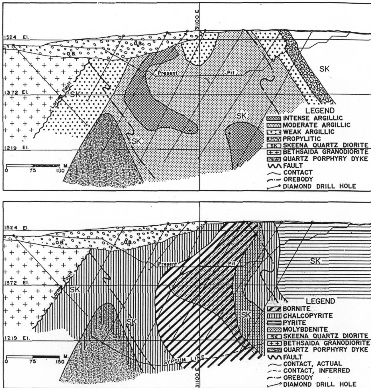
FIGURE 7 — Section A-A', looking north, showing: (a) zonation of hydrothermal alteration and (b) sulphide mineralization.
