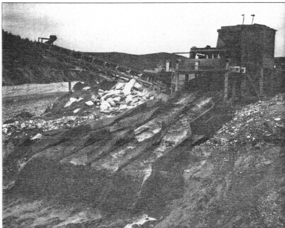
Sluice box where placer gold is concentrated, Klondike mine, Yukon Territory.
