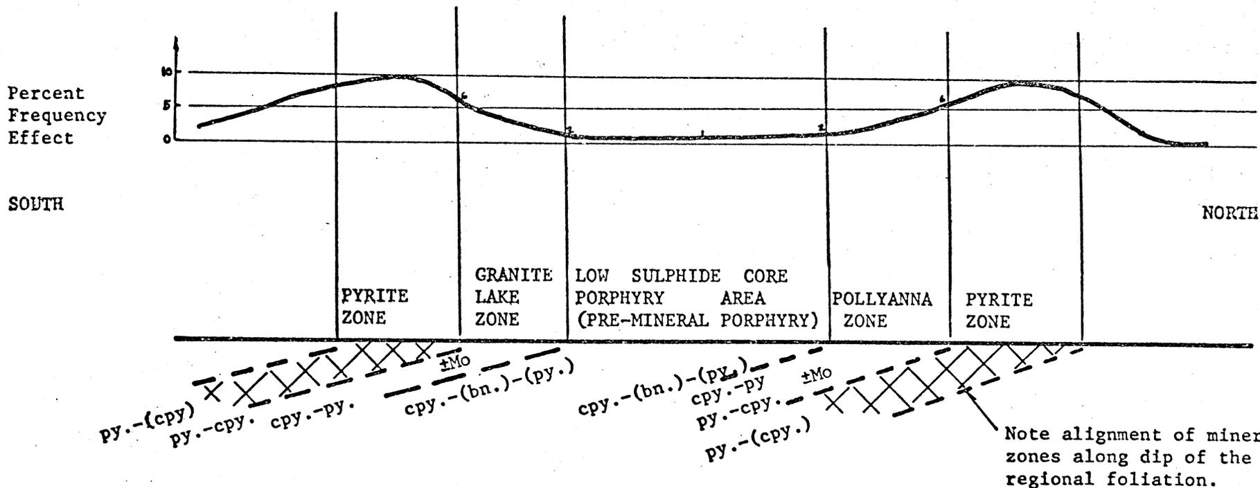
FIGURE 19: Diagrammatic North - South Cross-Section Of The Pollyanna And Granite Lake Zones Showing The Relationship Of I.P. Response, Primary Sulphide Mineral Zoning, And Location Of The Respective Open Pits. (py, = pyrite, cpy. = chalcopyrite, bn. = bornite, Mo = molybdenite, brackets indicate minor amount, if no brackets then both minerals are present in approximately equal amounts.)
