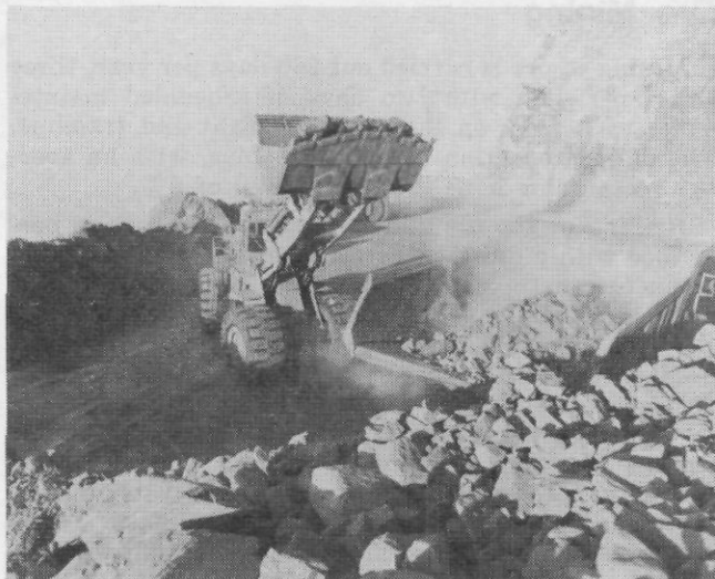
FIGURE 5—Caterpillar 992 front-end loader cleaning catchments to avoid rock spills onto the ore faces below.
