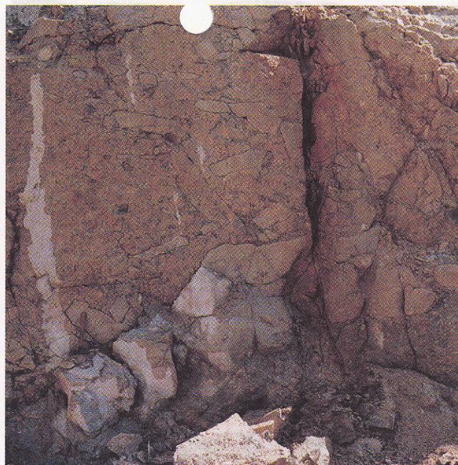
FIGURE 6. Northeast collapse breccia. Note slabs of QFP with rinds of black chalcidony “floating” in rhyodacite rubble. Bell mine, 2340 bench.
