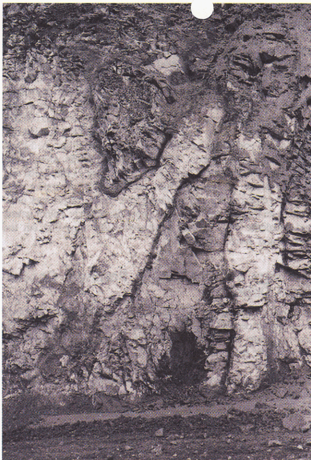
FIGURE 5. Post-stockwork QBFP/QFP dikes (light grey) intruding shattered core BBFP (dark grey). Note baked selvages along contacts and “sugar cube” jointing in BBFP.
