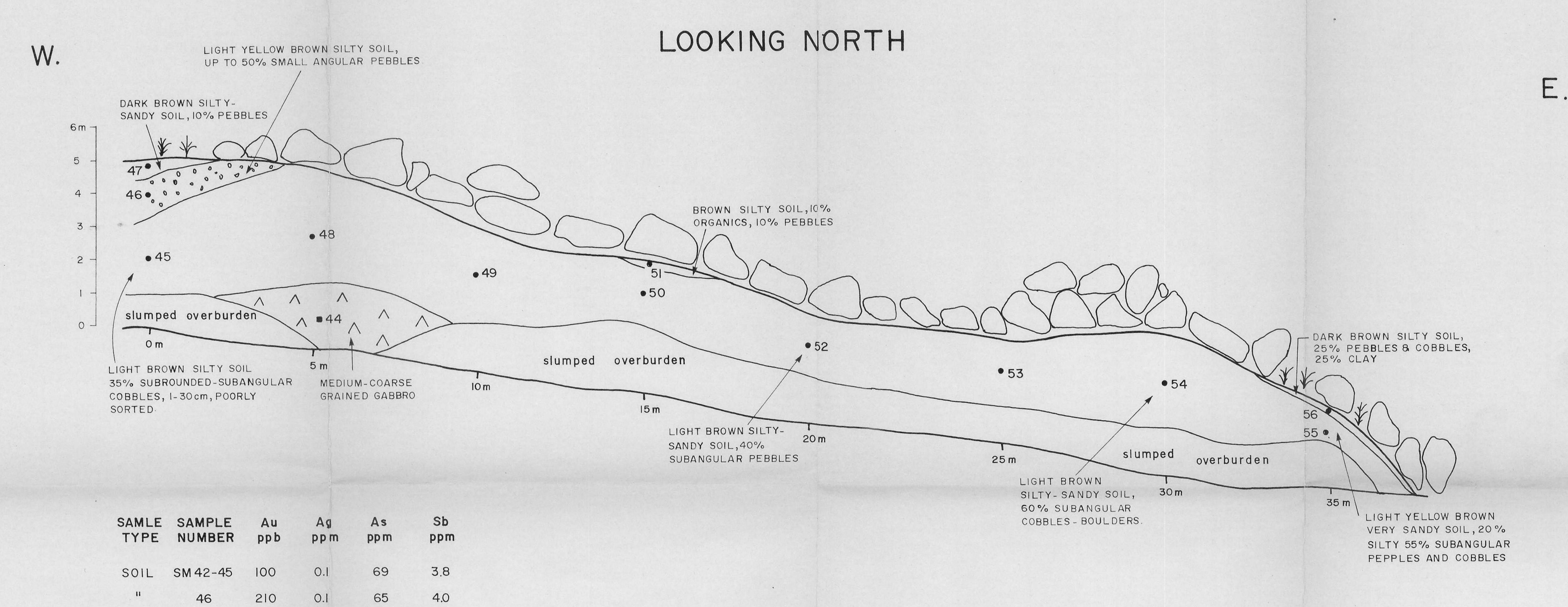
NOTE: Soil samples were taken every 5 m across the trench and at every different horizon present. This soil trench was put in to follow up a 1982 soil sample, DM-97, of 3250 ppb. Au. The trench cut through an area of landslide debris.
