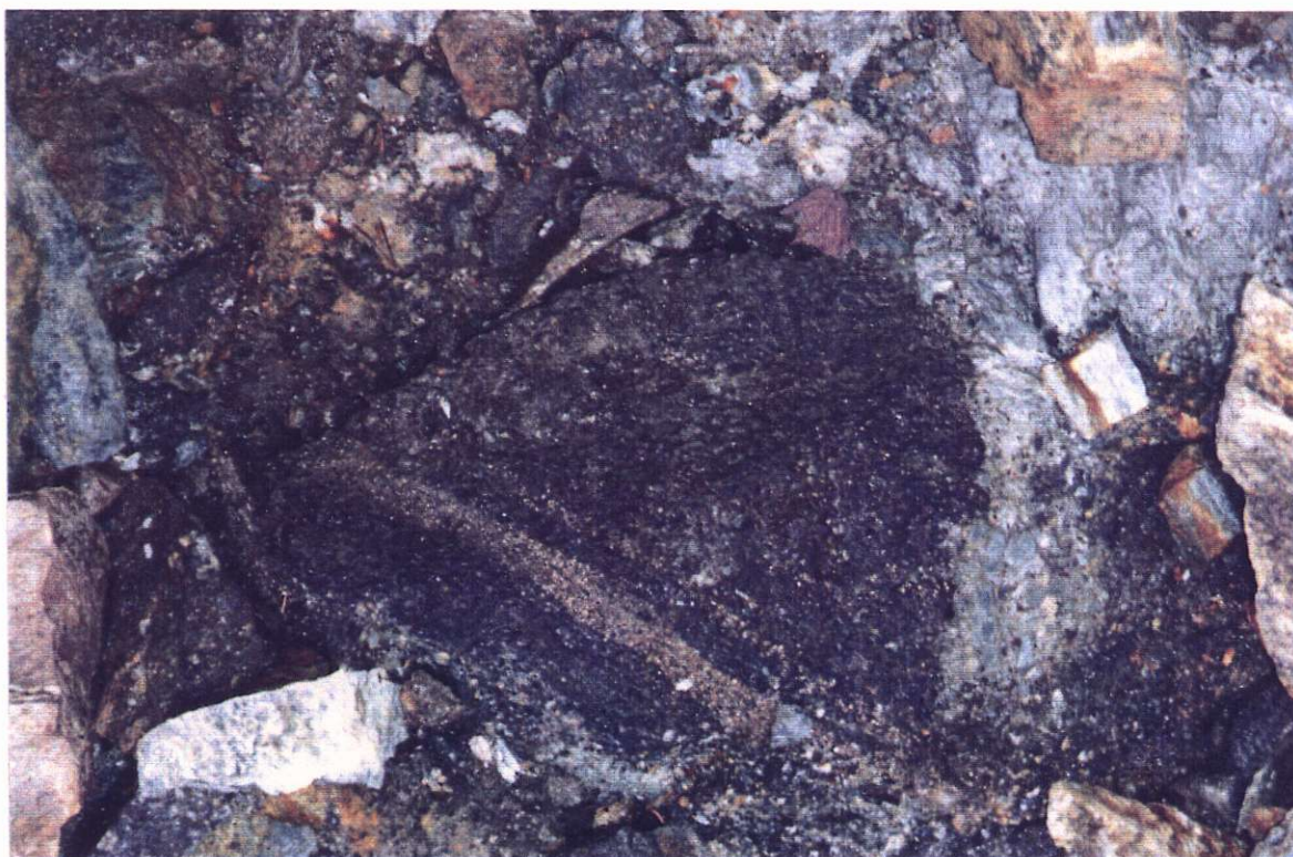
recrystallized banded (?) sphalerite + pyrite + chalcopyrite + barite mineralization
