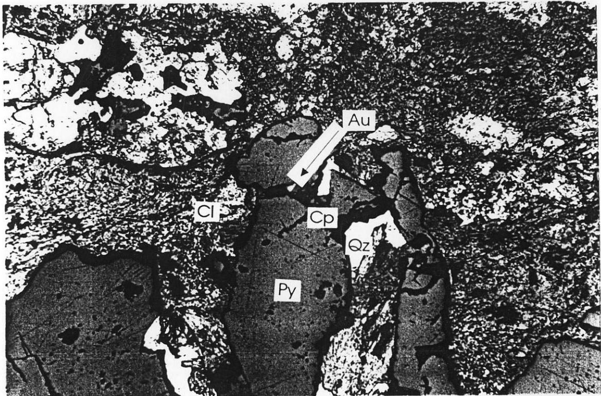
Plate 6.2. Broken pyrite grains in a matrix of Fe - chlorite grains, quartz and minor sericite. Gold occurs with chalcopryite in fractures in pyrite. Sample is from KS-125 286.0 m, Figure 4.2. Field of view is 1.25 mm. Legend: Au - Gold, Cl - chlorite, Cp - chalcopryite, Py - pyrite, and Qz - quartz.
