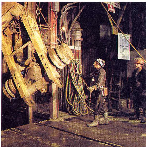
In order to remove or add to the more than 100 pieces of equipment used underground in the H-W Mine, the equipment has to be taken apart and raised or lowered down the shaft under the cage. Here Terry Ryan and Rick Schultz bring a truck to surface.
