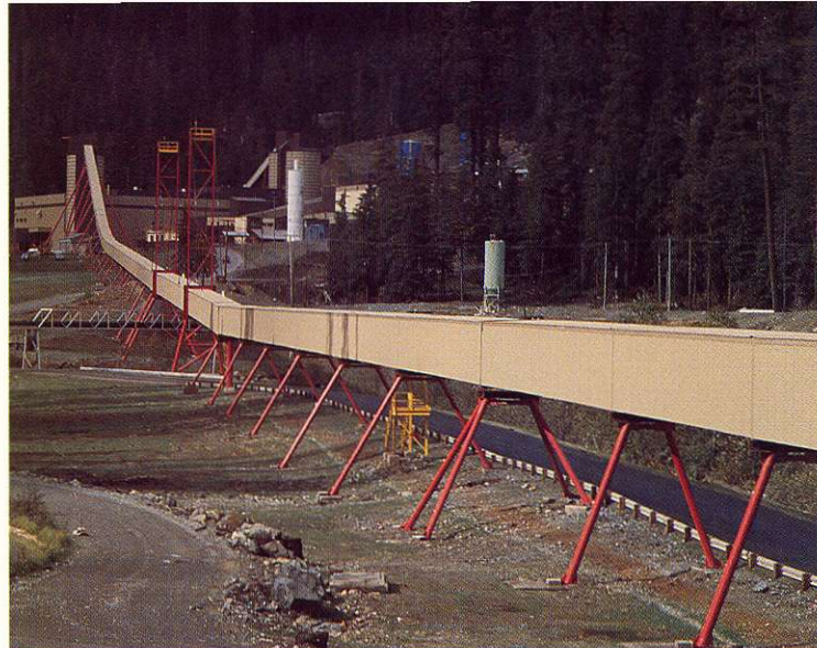
Mile-long conveyor transporting ore to silos and mill in background.
