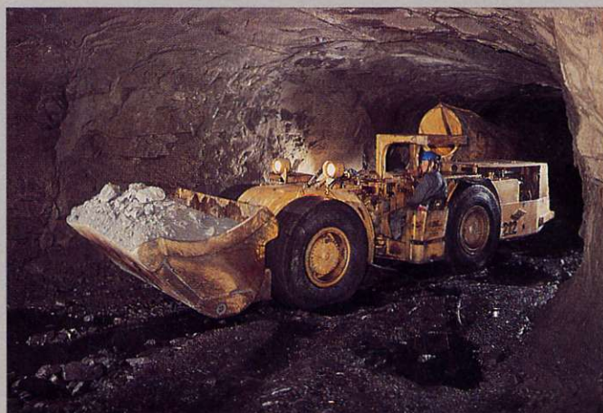
Underground at HW: Scooptram transporting ore from draw point to orepass.
