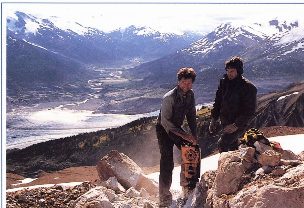
FIELD CREW DRILLS HOLES FOR DYNAMITE TRENCHING TO EXPOSE GOLD-BEARING FELSIC VOLCANIC ROCKS ON THE DELTA PROPERTY, SULPHURETS AREA, BRITISH COLUMBIA
