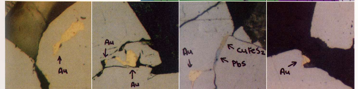
A gold grain 50 µm in length is encapsulated in pyrite. A 25 µm gold grain is intergrown with pyrite. Several gold grains up to 10 µm, occur along fractures with chalcopyrite (dark yellow) and galena (silver-grey). A 7.5 µm gold grain occurs on the margin of a pyrite crystal.
