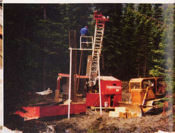
Pulling drill rods for the next phase of drilling on Bonanza Ledge during the winter work program on the Cariboo Gold Project.
