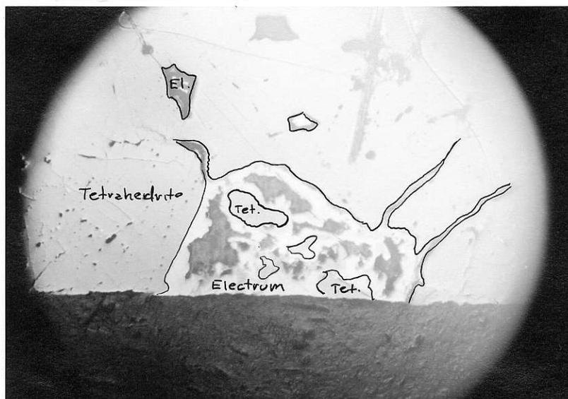
FIGURE 10 - Electrum replacing tetrahedrite, & electrum filled fractures in tetrahedrite.
