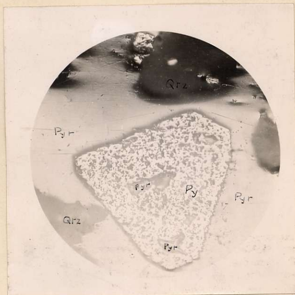
Fig.9 Centrifugal replacement (?) of pyrite (Py) by pyrrargyrite (Pyr)
