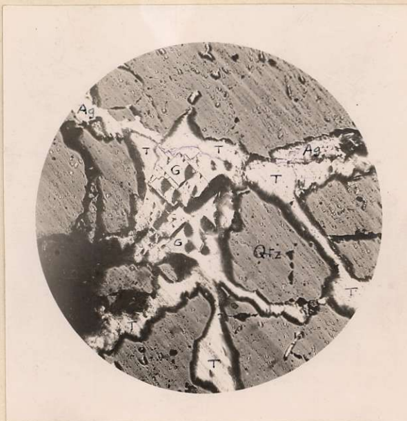
Fig. 10 Galena (G), Tetrahedrite (T) and native silver (Ag) in a veinlet.
