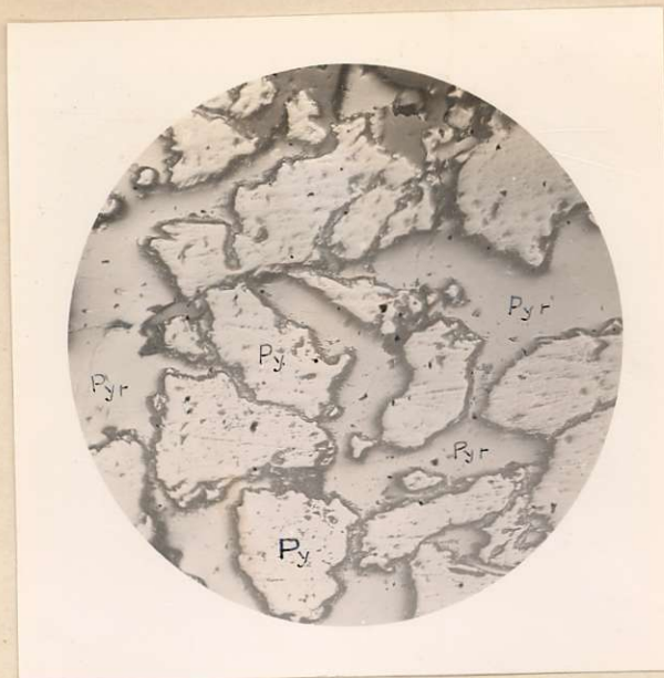
Fig 8 Residuals(?) of pyrite (Py) in pyrrargyrite (Pyr)
