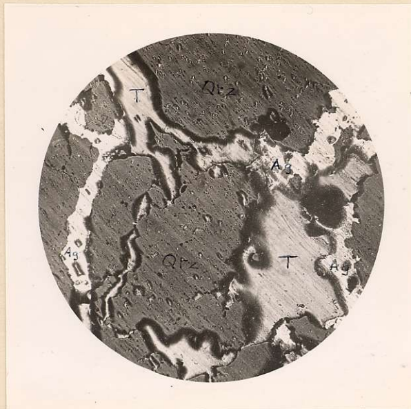
Fig: 12. Native Silver (Ag) occupying the same fracture as Tetrahedrite (T).
