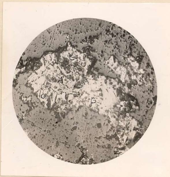
Fig. 11 Galena (G) later than Argentite (A) in a veinlet.
