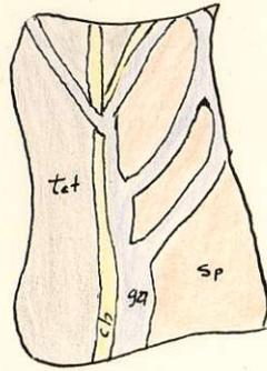
Galena veining through and replacing sphalerite, chalcoppyrite, and tetrahedrite.
