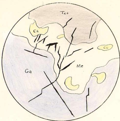
Anglesite veinlets following cleavage planes in galena, meneghinite, and tetrahedrite.
