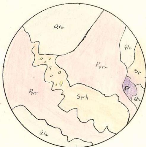
Sphalerite veining through pyrrhotite
