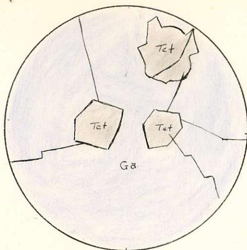
Simultaneous deposition of galena and tetrahedrite or tetrahedrite may be replacing galena along cleavage planes.
