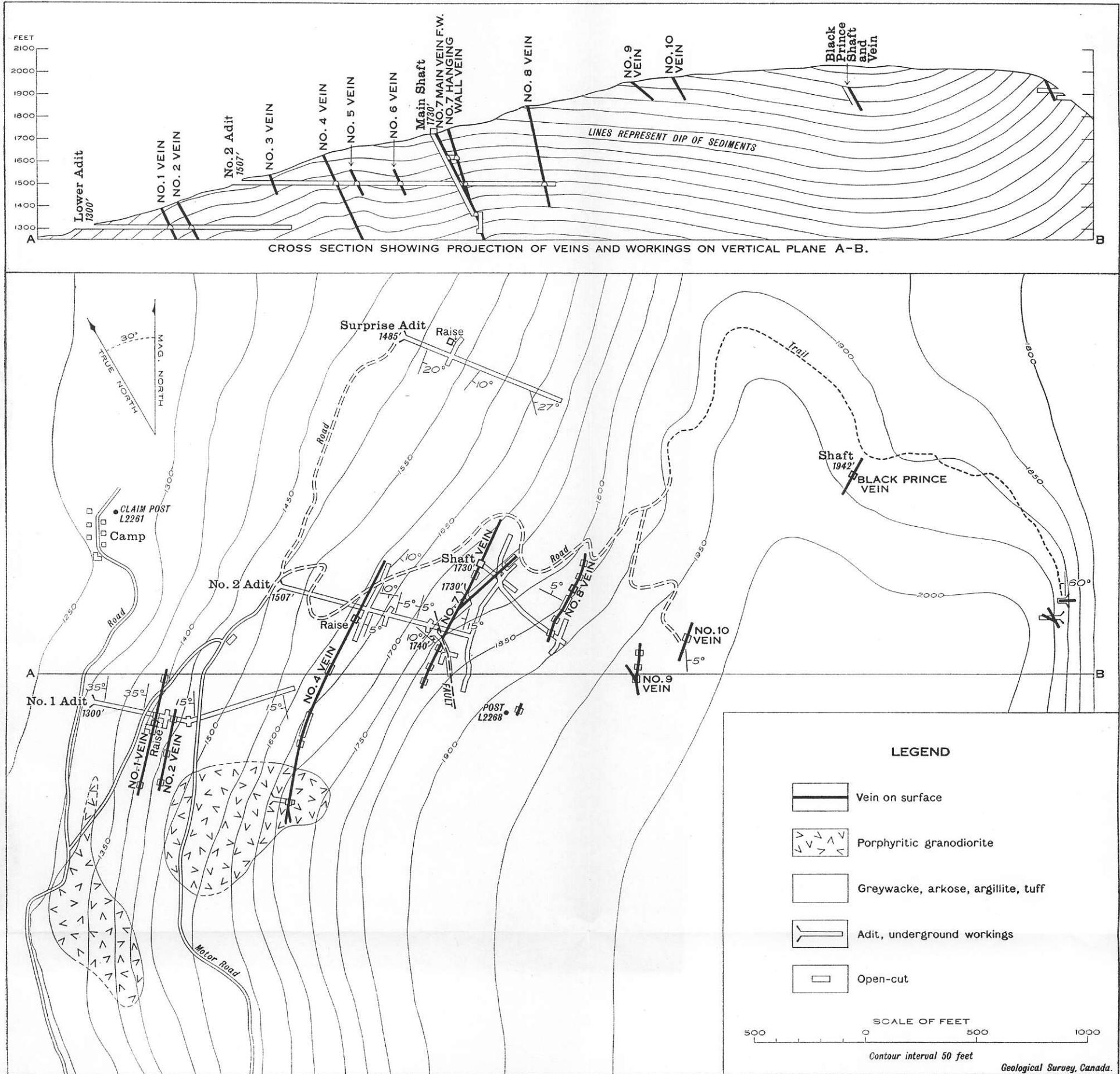
Figure 5. Plan and section of part of the Silver Standard property.
