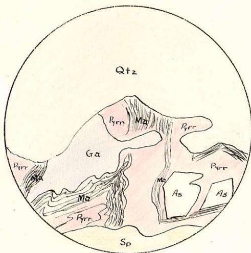
Lamellar marcasite replacing
