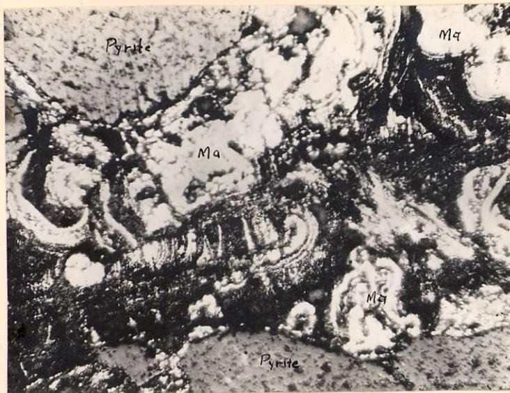
Irregular composite lamellae of marcasite showing complete replacement of pyrrhotite around pyrite grains.
