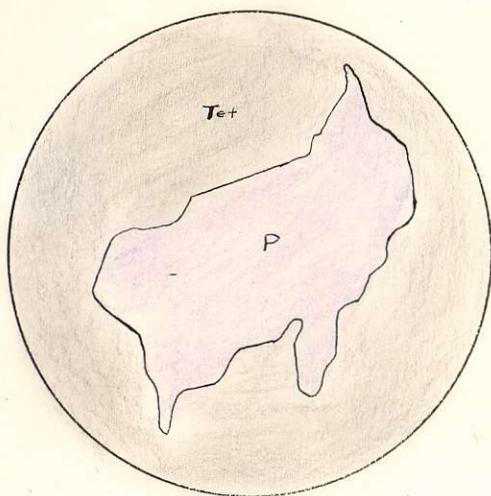
Pyrargyrite in typical isolated mass in tetrahedrite.
