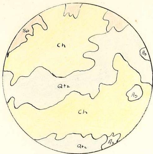
Chalcopyrite as large masses associated with quartz and extending into sphalerite. Chalcopyrite and quartz show corrosion of arsenopyrite.
