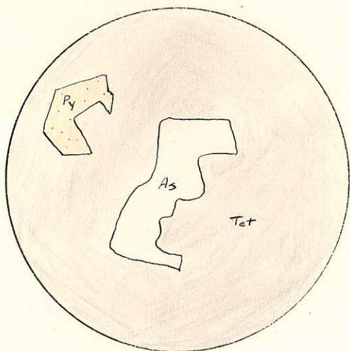
Corrosion of euhedral arsenopyrite and pyrite by tetrahedrite.
