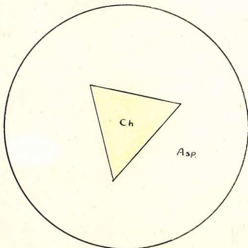
Idiomorphic chalcopyrite crystal replacing euhedral arsenopyrite grain from core outward.
