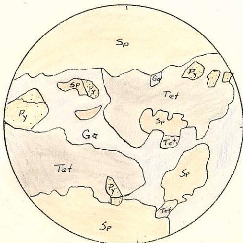
Galena and associated tetrahedrite veining through sphalerite.
