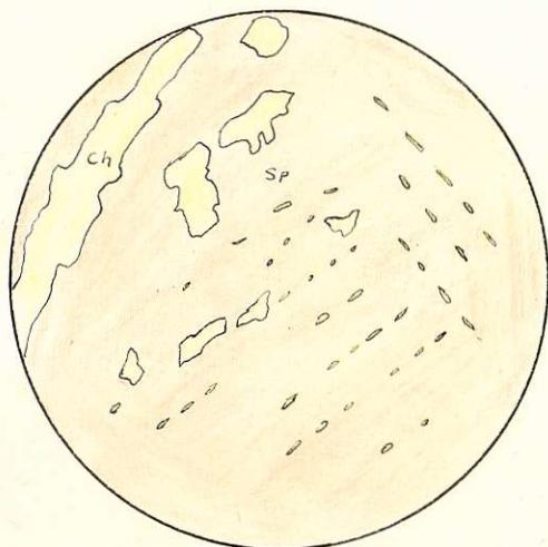
Exsolution chalcopyrite along crystallographic planes of sphalerite.
