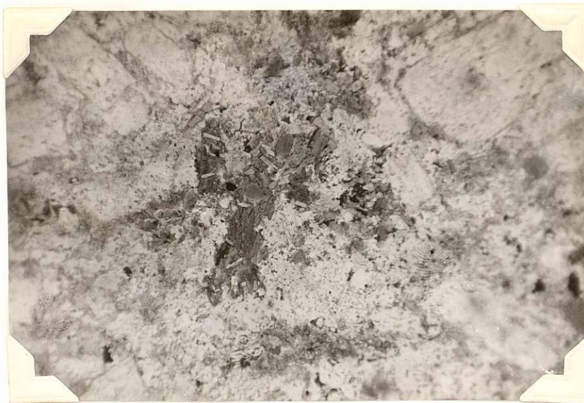
Fig. 7. Biotite, Feldspar (both as phenocrysts) and a matrix of sericite. Plain light. Hole # 6 - 70'. X 30.
