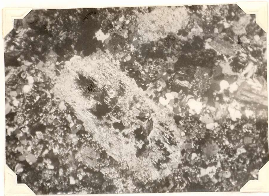
Fig. 3. Partially sericitized feldspar phenocryst. Crossed nicols. Hole # 6 - 70'. X 40.
