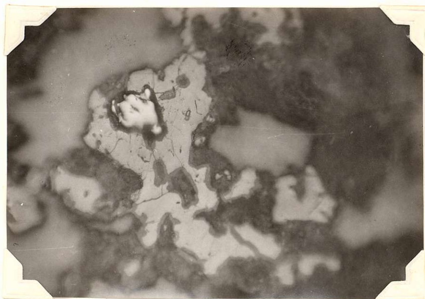
Fig. 12. Chalcopyrite with rim of digenite. Plain light. Hole # 3 - 70'. X 250.
