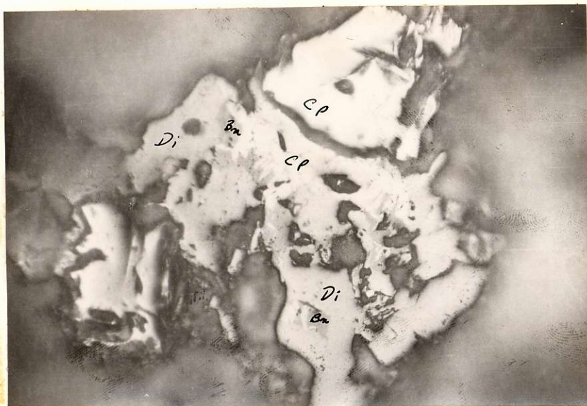
Fig. 14. Chalcopyrite and bornite partially replaced by digenite. plain light. Hole # 87 545'. X 75.
