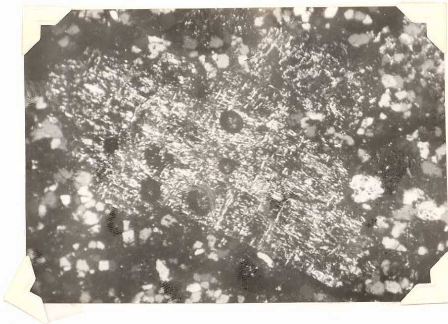
Fig. 4. Completely sericitized feldspar phenocryst, note that the sericite is developed parallel to the feldspar cleavage. Crossed nicols. Hole # 3 - 70'. X 30.
