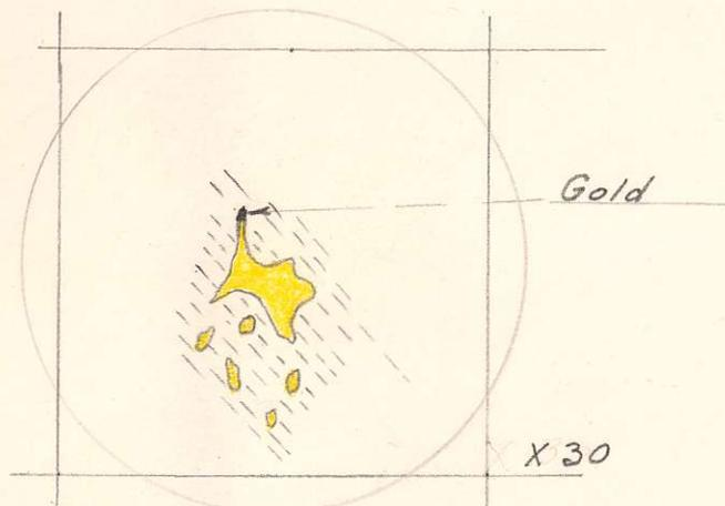
Gold at point of contact of sphalerite and pyrite.
