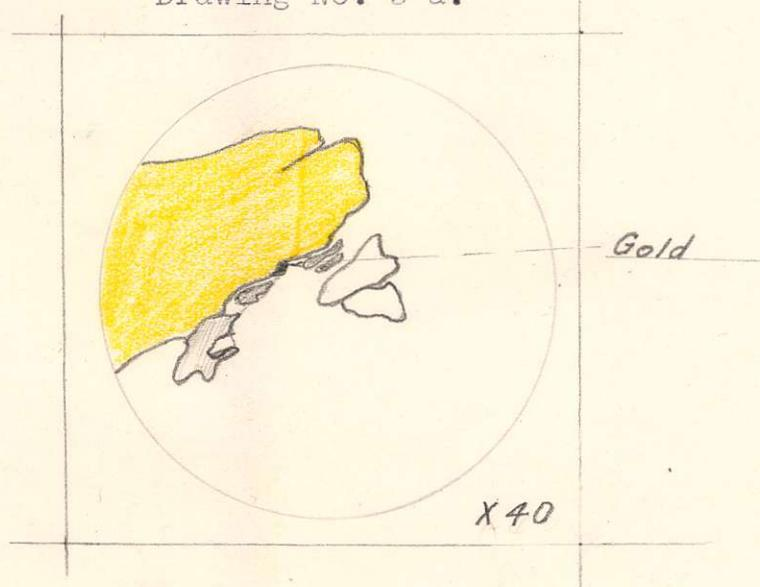
Gold on the edge of a piece of pyrite; probably the contact between pyrite and galena or sphalerite.
