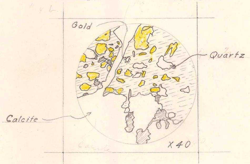
Very fine gold particles in sphalerite around a quartz inclusion.
