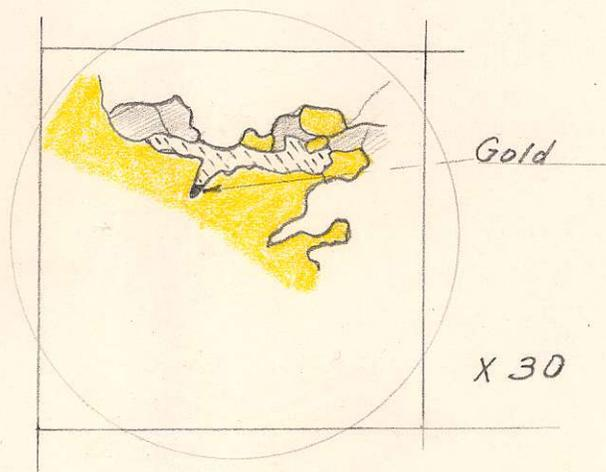
Gold at the head of a channel of sphalerite into pyrite.
