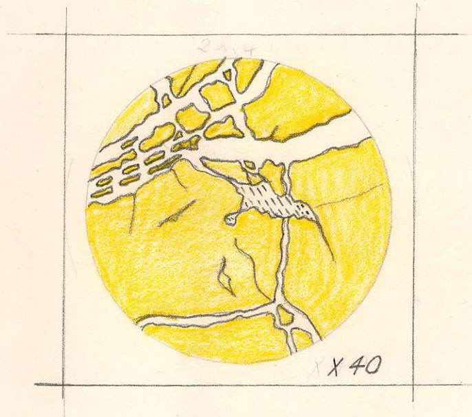
Massive pyrite, showing its fractured nature.
