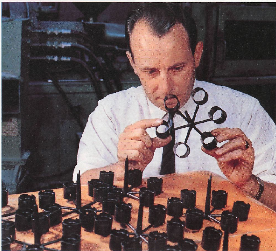
43 Asbestos-reinforced polypropylene, a new composite material, moulded to form lamp-holders.
