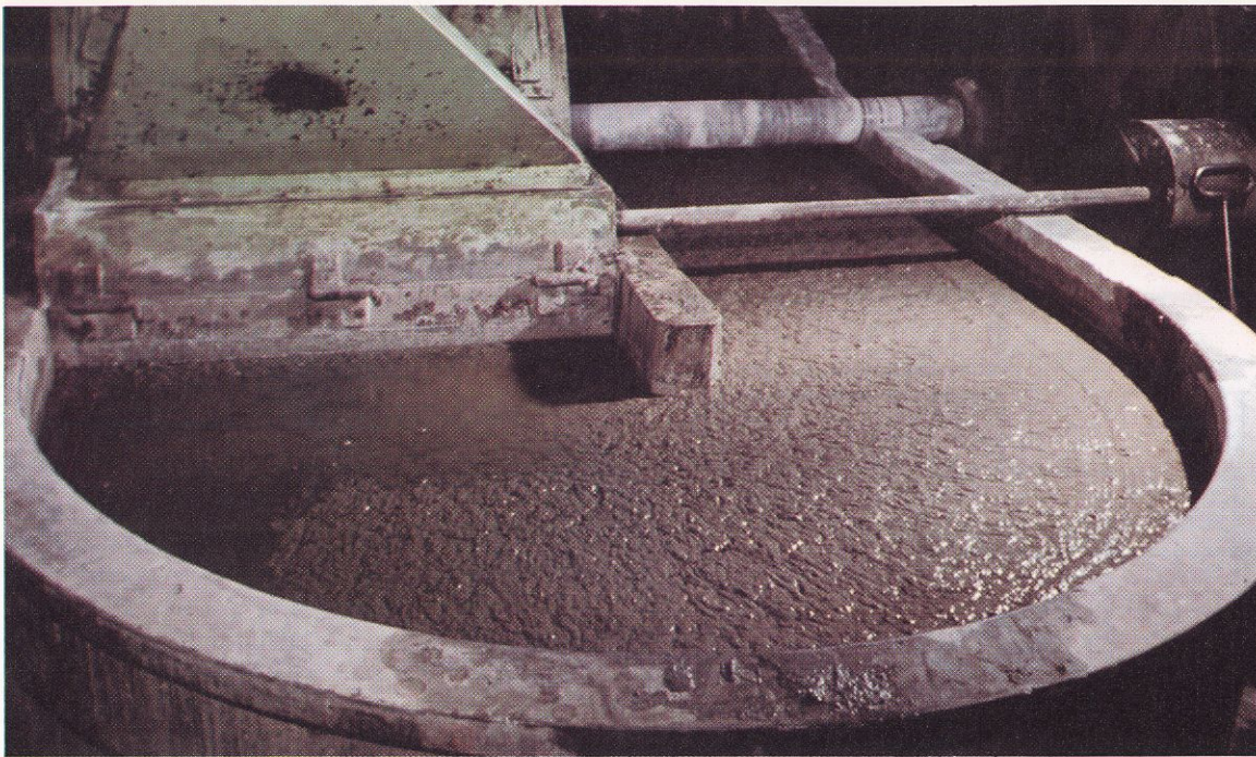
31 Asbestos fibres and cement are mixed with abundant water in the beater to form a homogeneous slurry.
