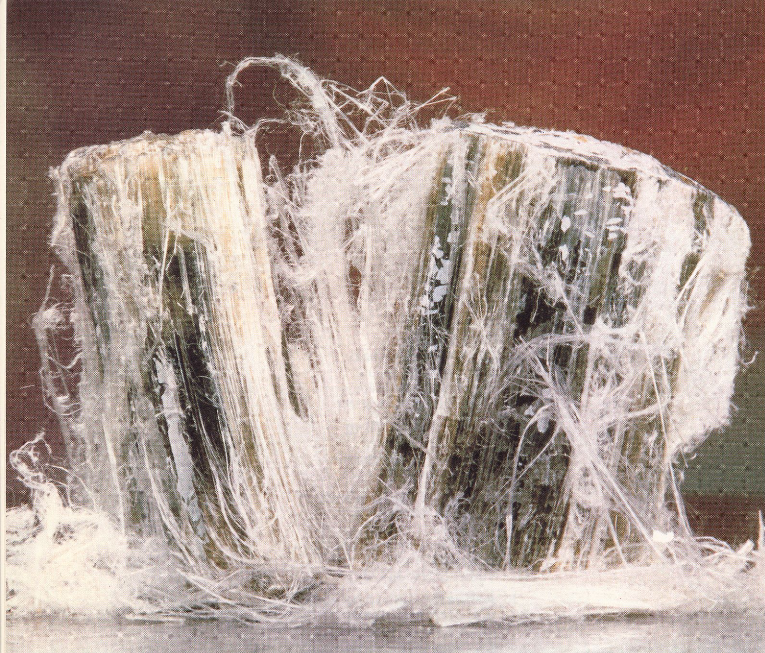
1 The solid green mass of chrysotile fibre breaks up into a "web" of white fibres. If what appear to be single fibres were further opened up, the ultimate single fibres would have a diameter in the region of one millionth of an inch. Photo: Derek Allen, Davyhulme.
