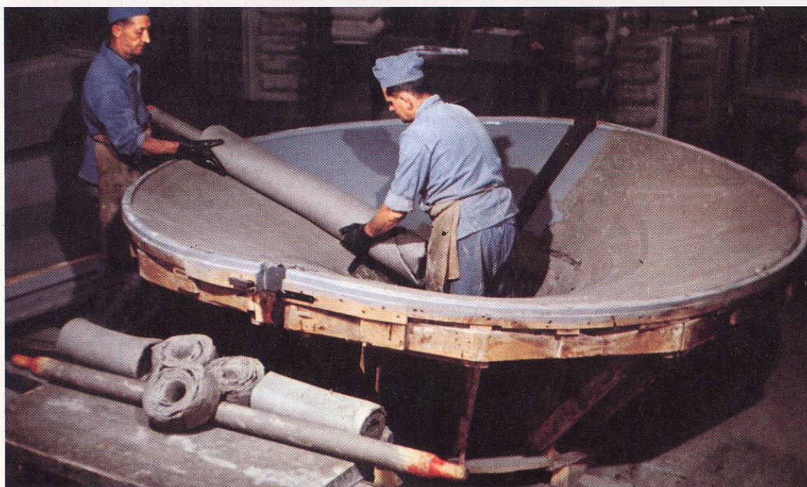
33 A mushroom head for use in reservoir construction is formed from freshly produced asbestos-cement sheets.
