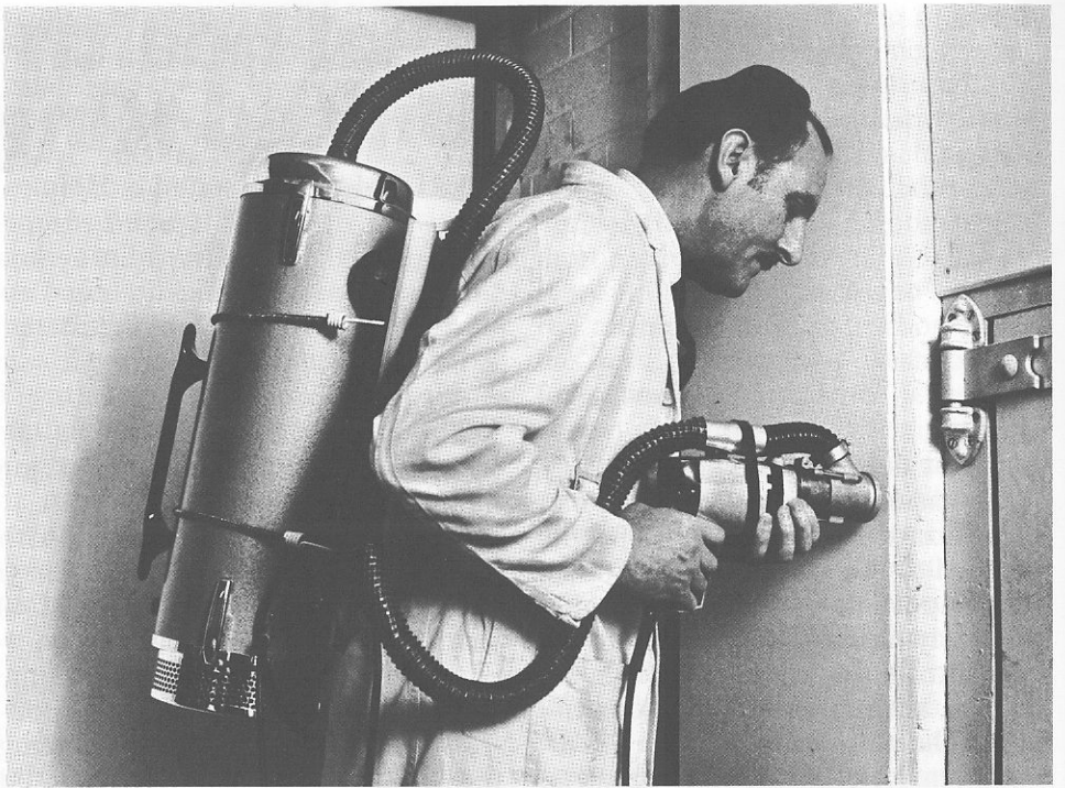
44 Portable suction equipment for use when drilling asbestos insulation board. Photo: Owen Lawrence, London.
