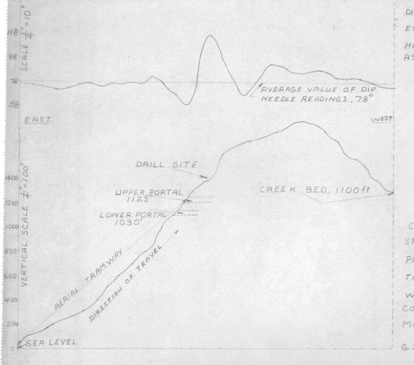
DIP NEEDLE READINGS FOR EVERY 100 ft OF ALTITUDE HORIZONTAL SCALE SAME AS BELOW
