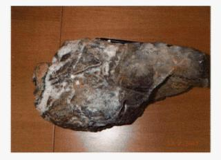
Figure 8 - Example of gold and silver rich vuggy quartz breccia vein from the 1870 level. Sample BD-40: 171 g/t gold, >100g/t silver.
