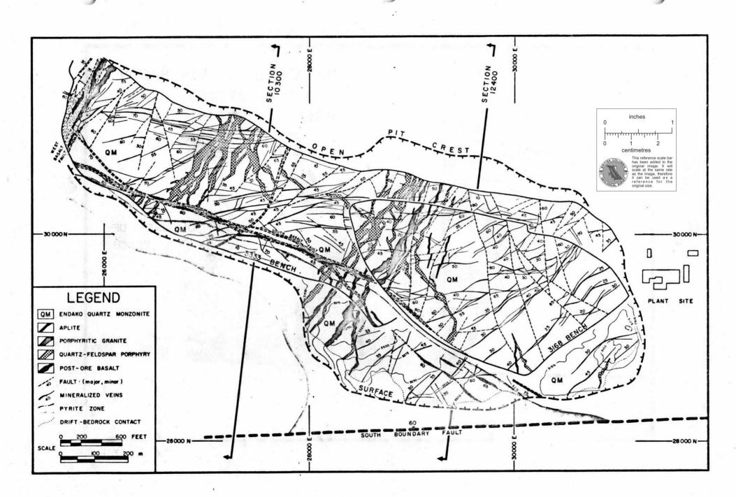
The ore minerals are intimately associated with quartz veining and occur in two types of veins: 1. as large four-inch to four-foot-wide veins in which molybdenite typically occurs as thin, closely spaced laminae, and 2. as fine fracture-fillings and veinlets in the form of stockwork. Orientation and limits of economic stockwork are controlled by major subparellel sets of south dipping and complementary flat-lying, southeasterly and northwesterly-dipping vein systems.
