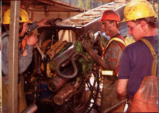
Diamond drilling from the portal in advance of the decline for the bulk sample program at the Bonanza Ledge Zone.
