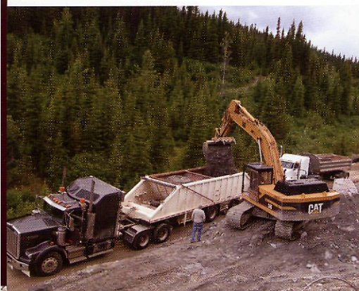
Loading mineralized material from Bonanza Ledge bulk sample for shipment to the Mount Polley Mill for processing.
