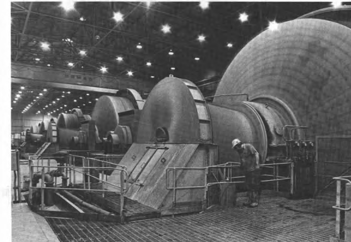
Six semi-autogenous grinding mills each process 300 tons of material per hour.
