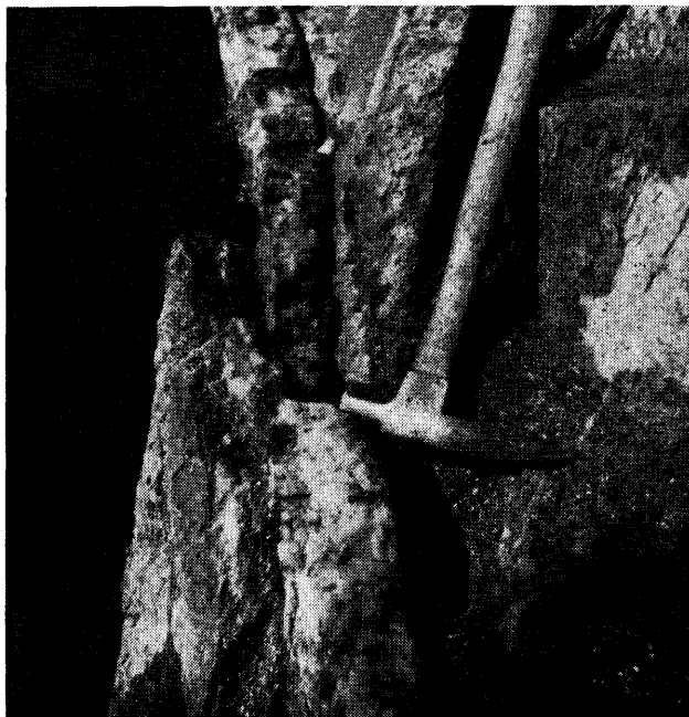
Gold-quartz vein in Tertiary quartz diorite at Faith lake on the Forbidden Plateau. Note comb texture and banding of the quartz and sulphides.
