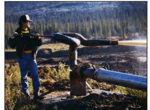
Queenstake uses water monitors such as this hydraulic set-up at Maysy May Creek to inexpensively remove thawed overburden from pay gravels.
