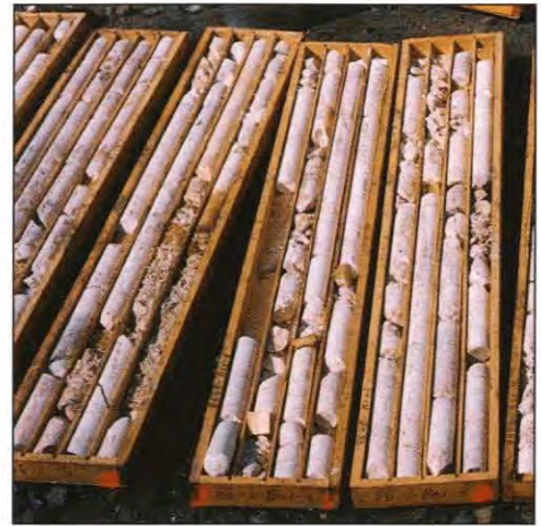
1986 diamond drilling on the east zone of the O'Connor River gypsum deposit indicated extensive gypsum reserves. A 1988 bulk sampling program is planned to demonstrate economic marketability of the gypsum.
