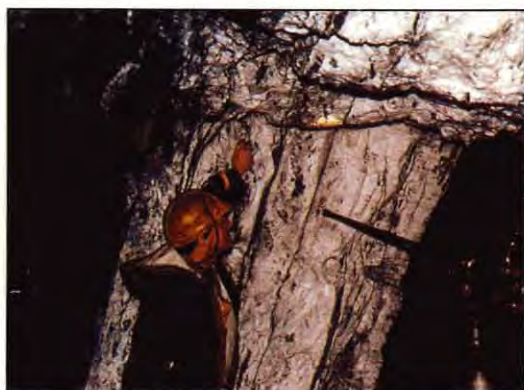
Gordon Gutrath, examines the drift face in the Big Croppings vein, a quartz vein which appears to be a typical Chichagof ore shoot.
