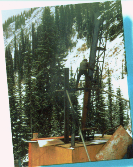
Diamond drilling a 2,000-foot hole from the 6,200-foot elevation to test the west extension of the Silvana main lode.
