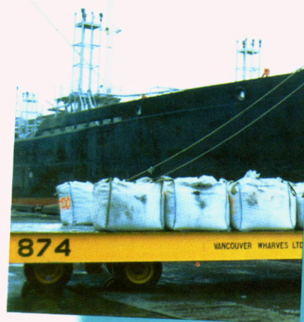
Bags of gold flotation concentrate prior to loading on a ship to Japan for smelting. Roughly 35% of the 18,000 ounces of gold produced at the Ptarmigan Mine was contained in the flotation concentrates.
