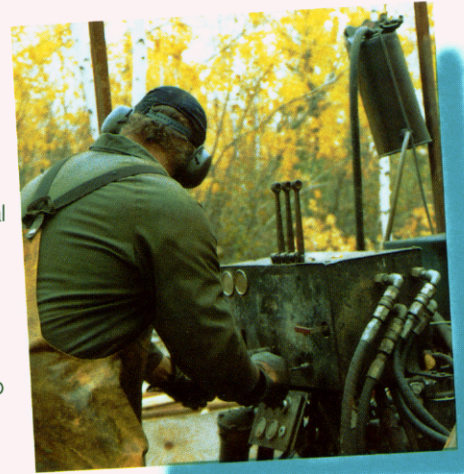
Contractor Tony Shearcroft diamond drilling the C Vein at the Parmigan Mine. The drilling indicated an ore reserve of approximately 70,000 tons grading 0.35 oz gold per ton above the 400-foot level. A decline to develop this ore body is currently proceeding.
