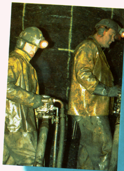
Miners George Mellen and Rick Gill drill off a drift round at the Silvana Mine.
