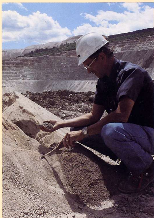
Geologist collects samples from the explosive drill holes prior to blast.
