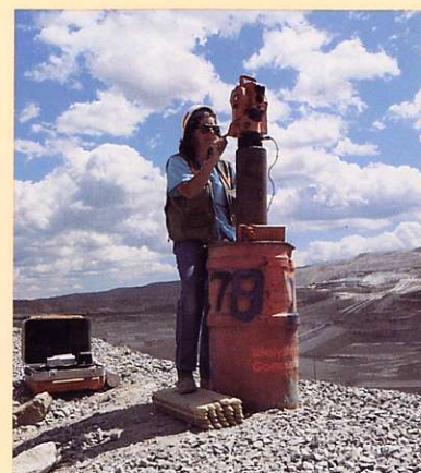
Surveyor takes geodimeter reading from atop the pit.
