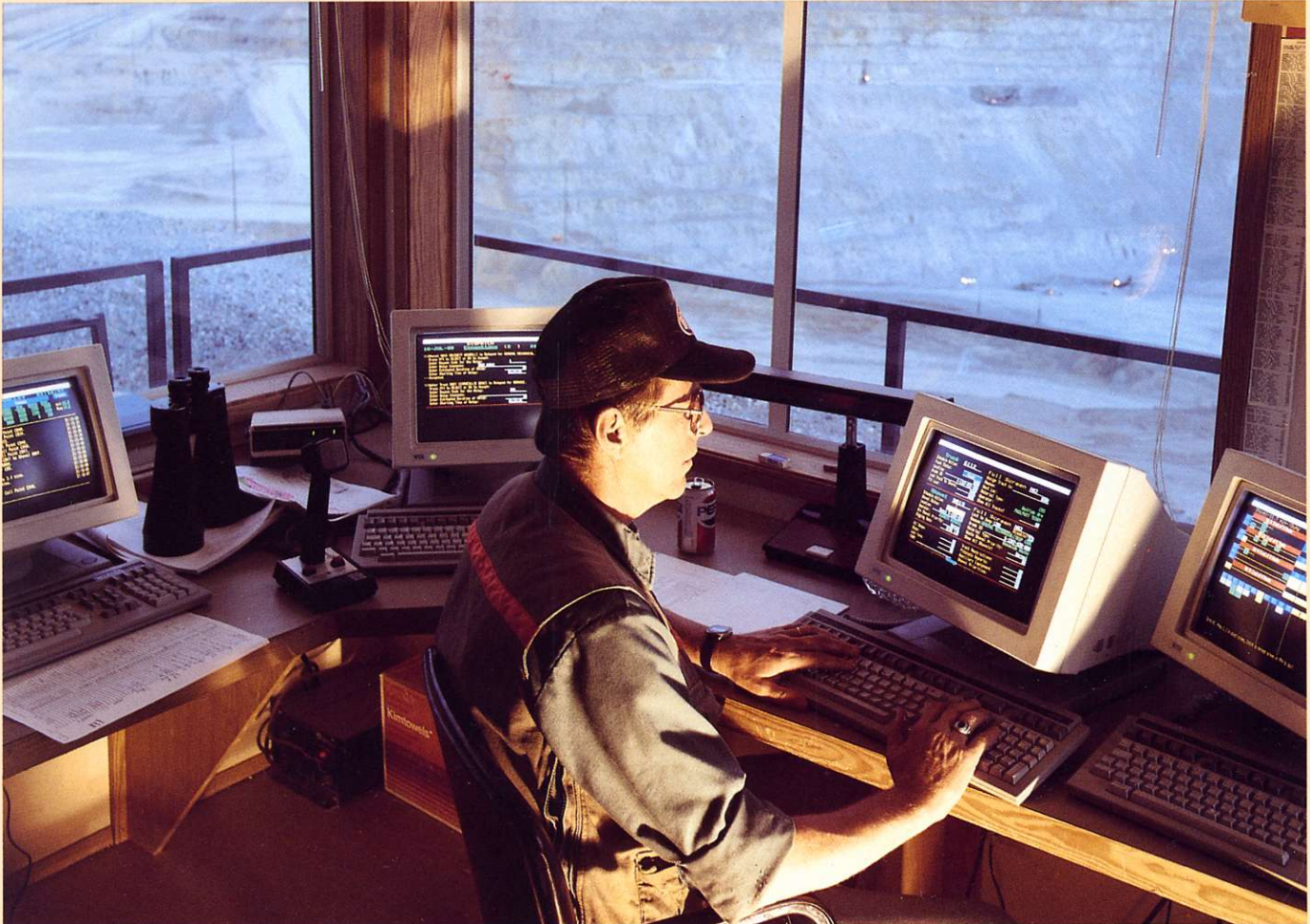
Through the use of computer electronics and a superior vantage point the Valley pit dispatch operator controls the movement of the haulage trucks.
