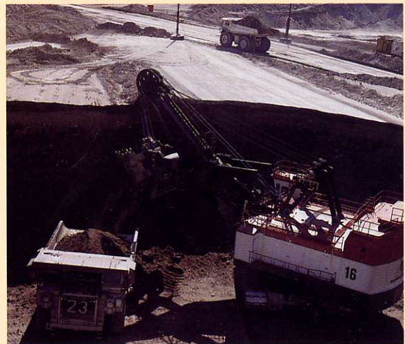
The team of shovels and trucks can move over 6000 tonnes of Valley ore an hour to the in-pit crushers.
