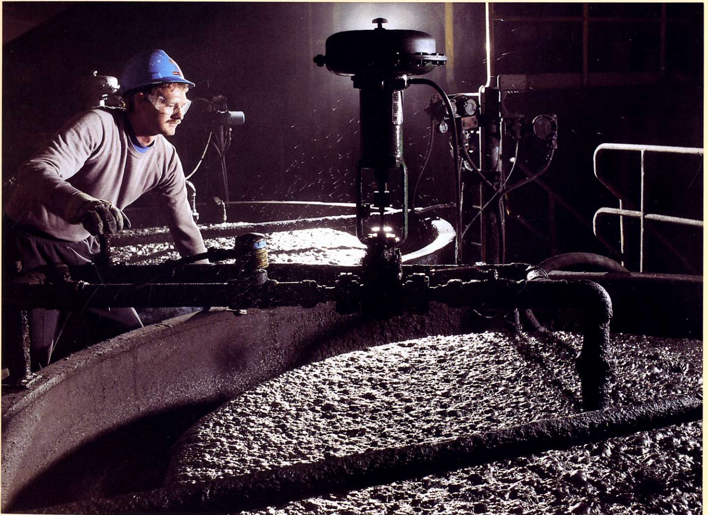
(Top left) The main control room in the Highland mill features the latest in computer technology. (Top right) Flotation operator adjusts air stream. (Above) Operator inspects the slurry in one of three column cells.
