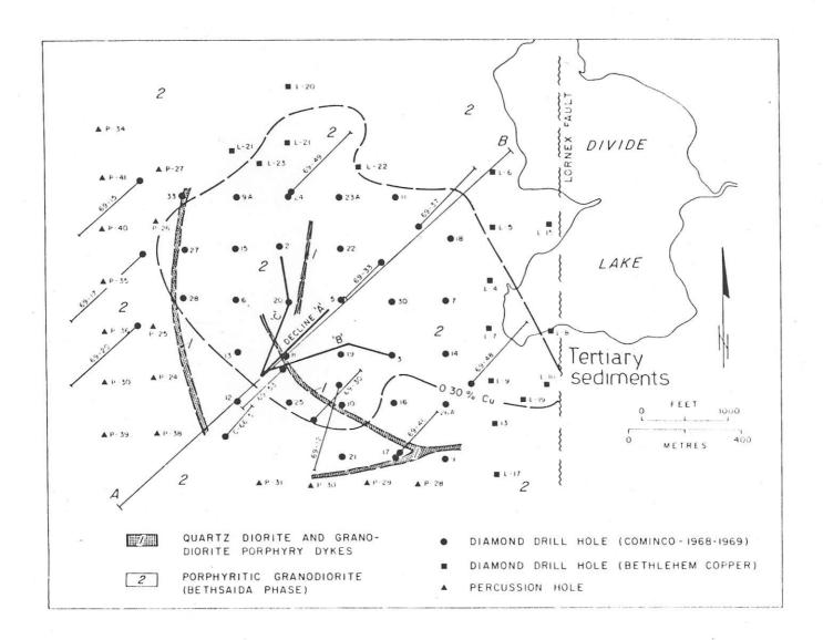
Figure 1. Geology of the Valley Copper deposit, showing distribution of drill holes studies, location of underground workings and location of vertical section A-B.
