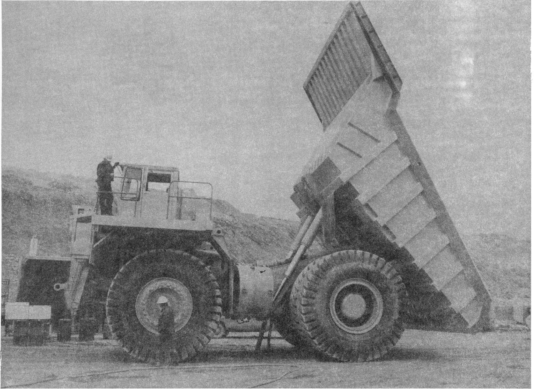
150-Ton Haulage truck at Lornex Mine.
