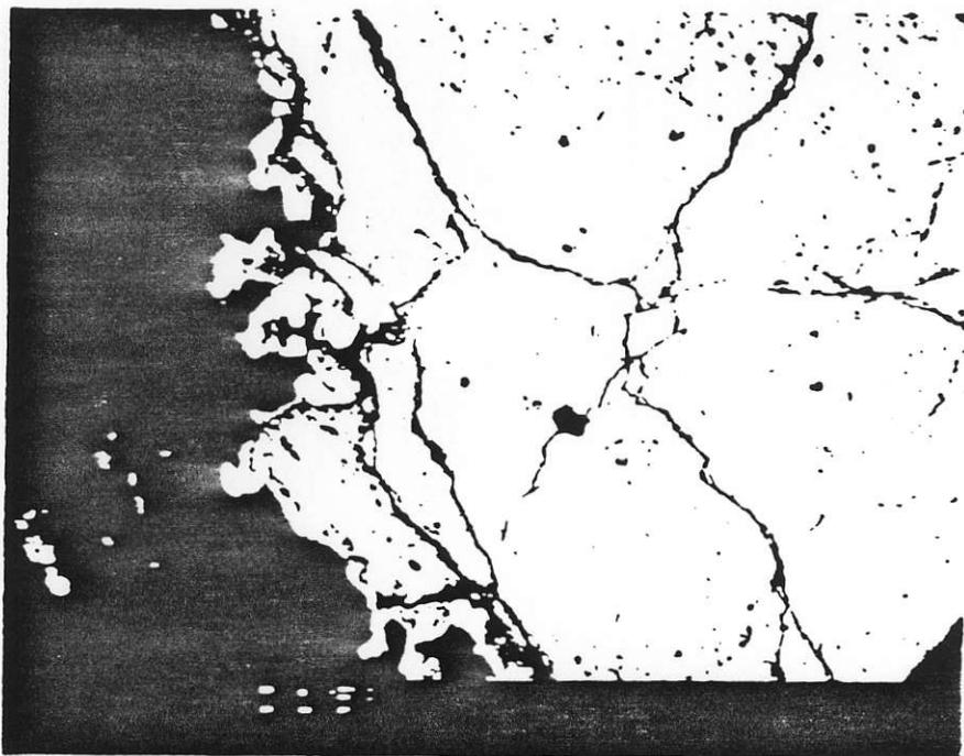
Sample CA-004 at 16X, BSE image. Black is quartz and the large grey mass is realgar rimmed with native arsenic at the left. Small (bright, nearly white) stibnite inclusions are just visible in the realgar.
