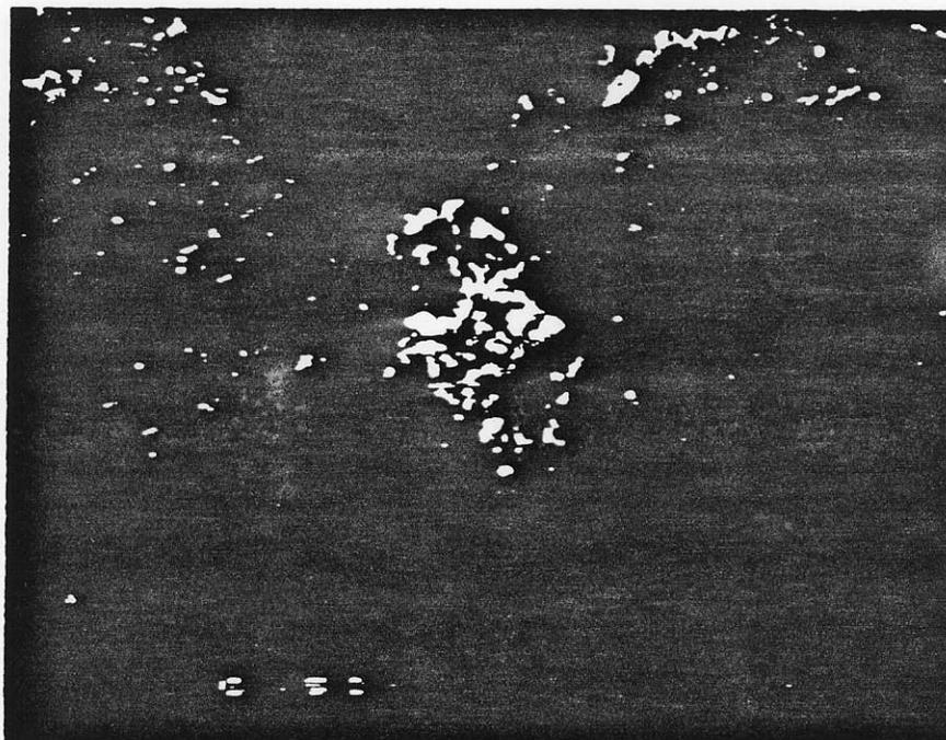
Sample CA-005 at 500X, BSE image. The black is gangue, dark grey is realgar. In the center is an irregular patch of (late) stibnite (grey) with a 4 $\mu$  white grain of cinnabar enclosed.
