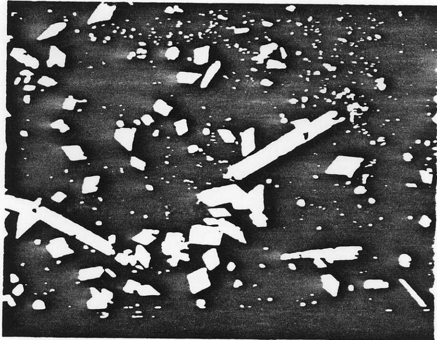
Sample CA-001 at 270X, BSE image. Field width is 500 $\mu$ . The white prisms and rhombic sections are arsenopyrite. Also visible are small (and greyer) spherules of pyrite (e.g. SE corner).
