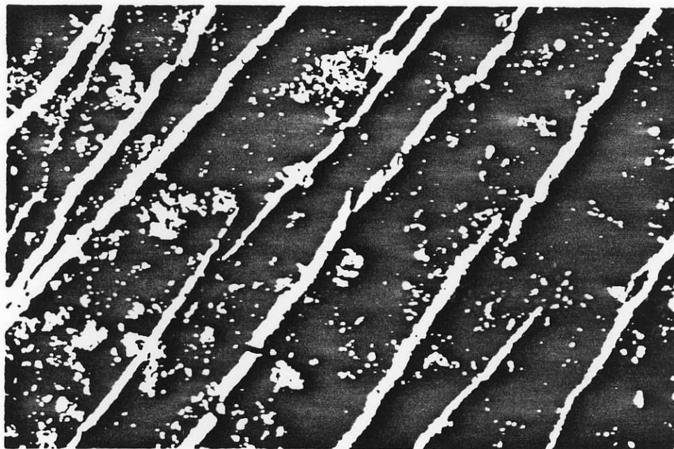
Sample CA-002 at 35X, Plane Polarized Light. Brown chert with numerous small fragments oriented about E-W. Black prisms of arsenopyrite lie in the chert. Numerous calcite veinlets in parallel cut obliquely across bedding. The length of a photograph at 35X represents 4mm.
