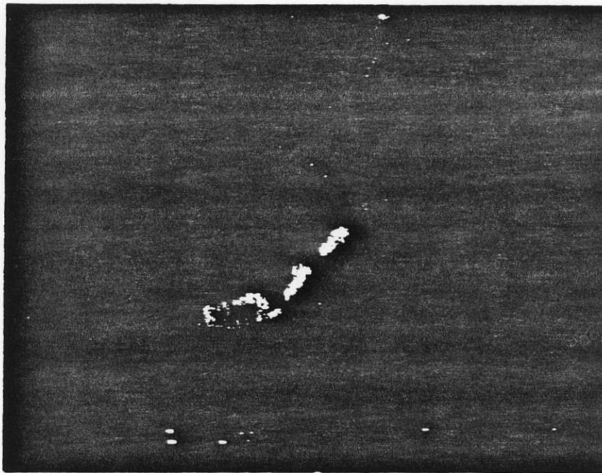
Sample CA-006 at 1500X, BSE image. The dull grey is stibnite with an irregular patch (slightly lighter grey, to the NE) of an unknown Pb-Ag-Sb sulfosalt). The lightest colored grains near the center are cinnabar.
