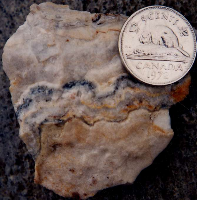
15. Banded silica with electrum + argentite, Ridge Zone, WOLF
