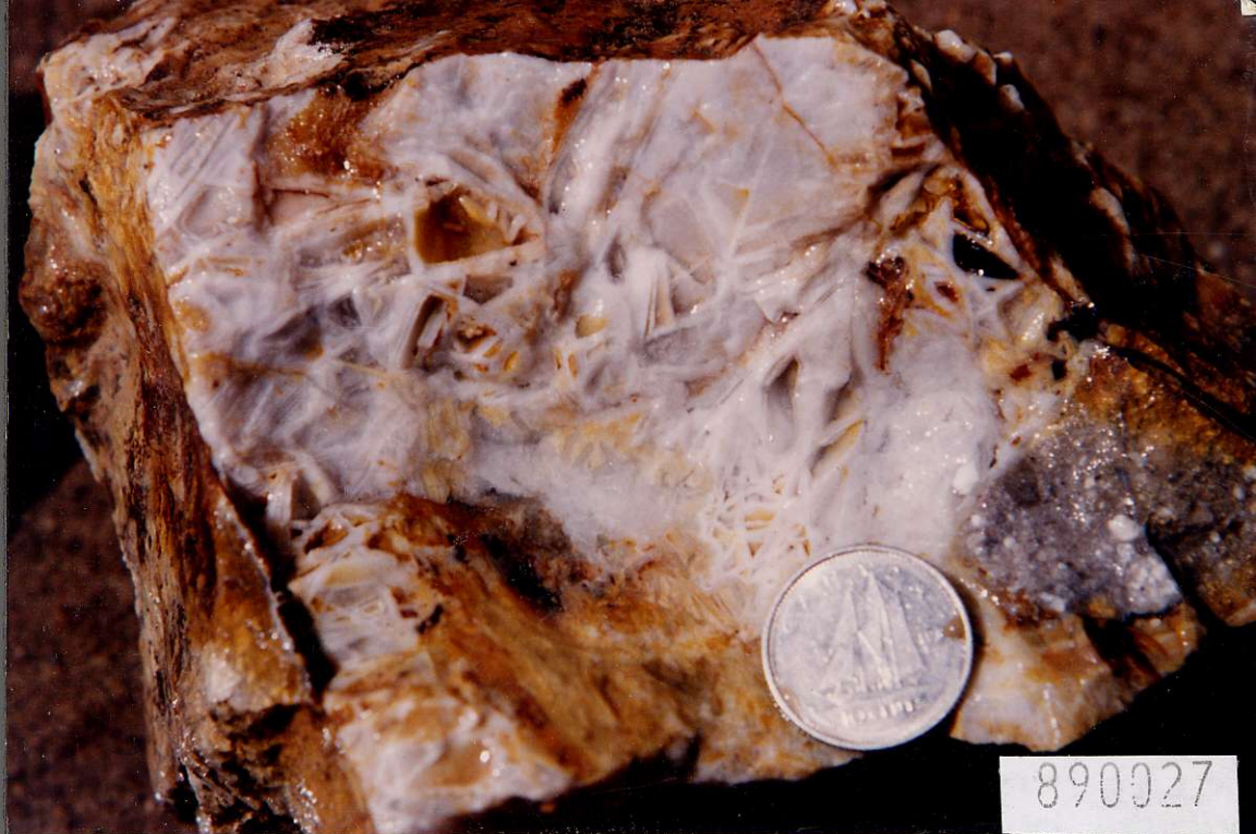
26. 'Angel' texture (barite blades replaced by silica), Ridge Zone, WOLF.
