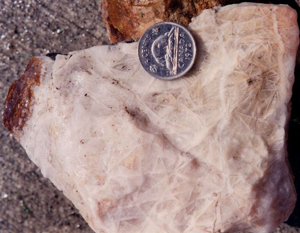
23. Coarse bladed silicified (ex-calcite) rock, WOLF . Characteristic high-level epithermal texture.
