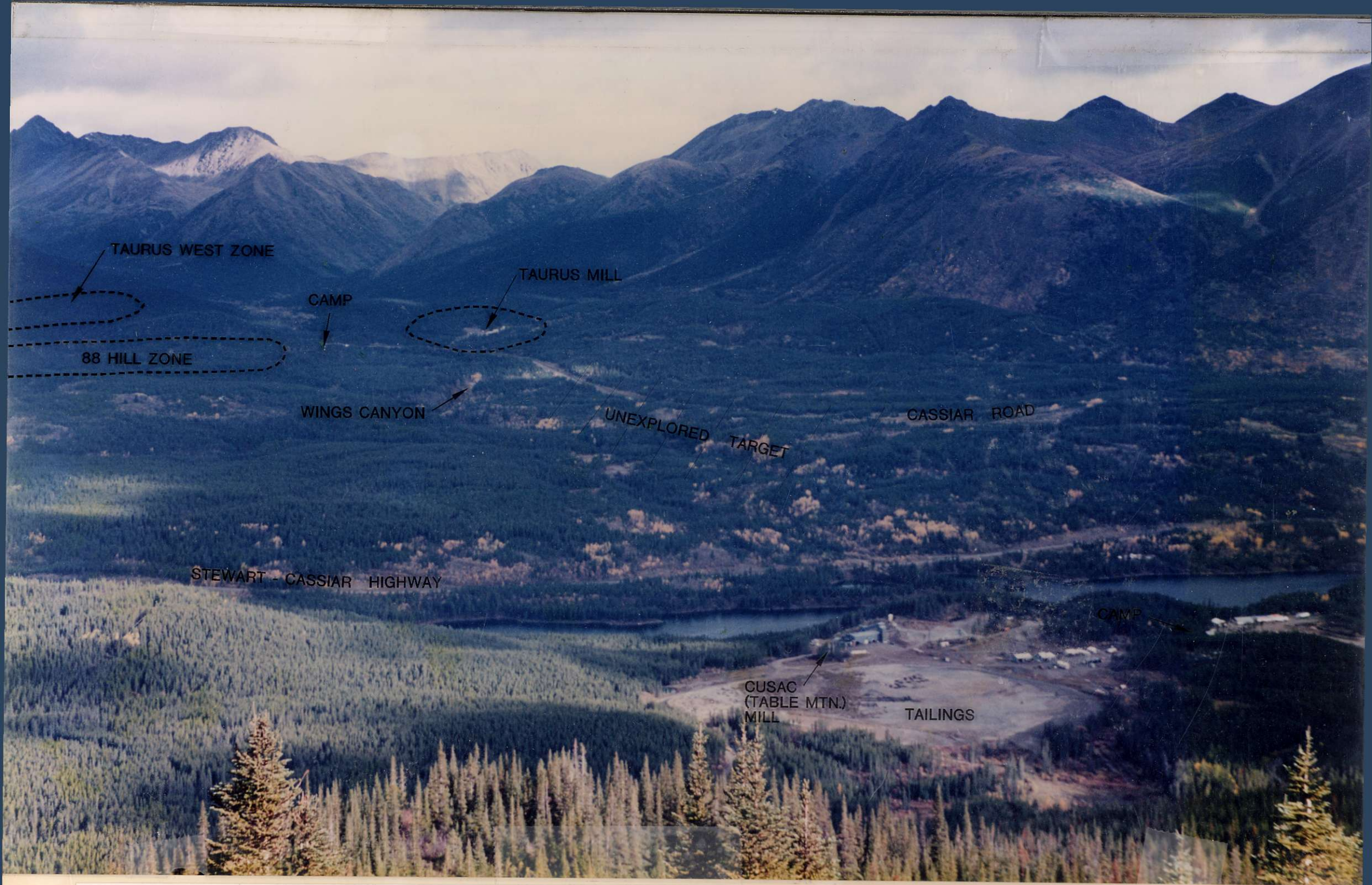
TAURUS. Looking northwest from Table Mountain over the Taurus deposit. A large tonnage, low-grade, open pit (potentially heap leachable) resource has been identified in the vicinity of the old Taurus, Sable and Plaza underground workings. The resource, estimated to be 130 million tonnes grading 0.95 g/t Au, is contained in three zones (88 Hill, Taurus West and BM) of carbonate-altered, pyritic volcanic flows and pyritic, gold-bearing quartz veins (previously mined by underground methods) that occurs between a hangingwall of basalt and a footwall of argillite.
