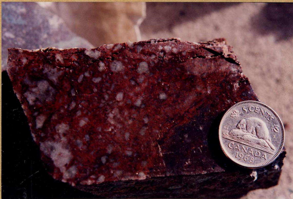
Red (C-2). Looking WNW toward Trench 4 area, where one of several north-westerly trending shear zones is exposed; b) close-up of auriferous, shear-controlled quartz-hematite vein, and; c) cut sample of quartz-hematite vein with disseminated native gold (bright specks) from high-grade section of Trench 4 that graded 3.59 opt Au over 5.5 m. See map in pocket for location.
