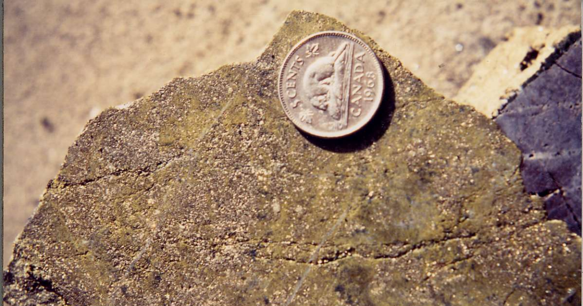
QR. Cut sample of auriferous chalcopyrite-pyrite bearing skarn from the Main zone pit.
