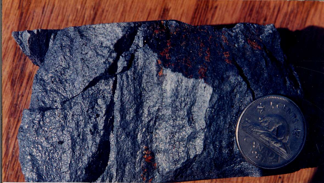
Massive stibnite and realgar, Contact Unit, 21A Deposit, Eskay Creek, DDH CA89-21: 60m.
