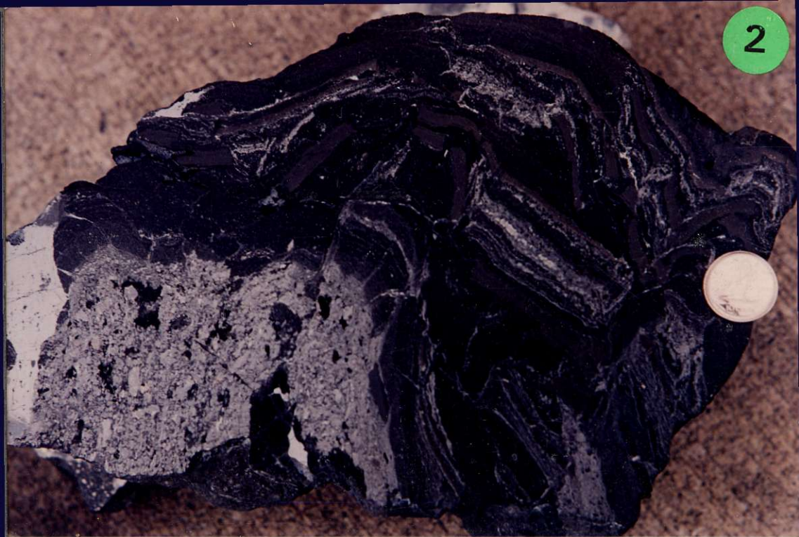
Disrupted massive sulphides (mainly sulphosalts, sphalerite, pyrite and younger stibnite) in argillite, 21B Zone, ESKAY CREEK .
