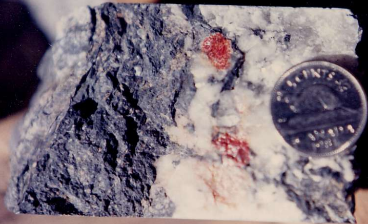
Realgar-quartz vein, Contact Unit, 21A Deposit, Eskay Creek, DDH CA89-23: 57m.
