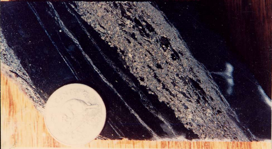
Bedded massive sulphides (sulphosalts and sphalerite) in argillite, 21B Zone, ESKAY CREEK.
