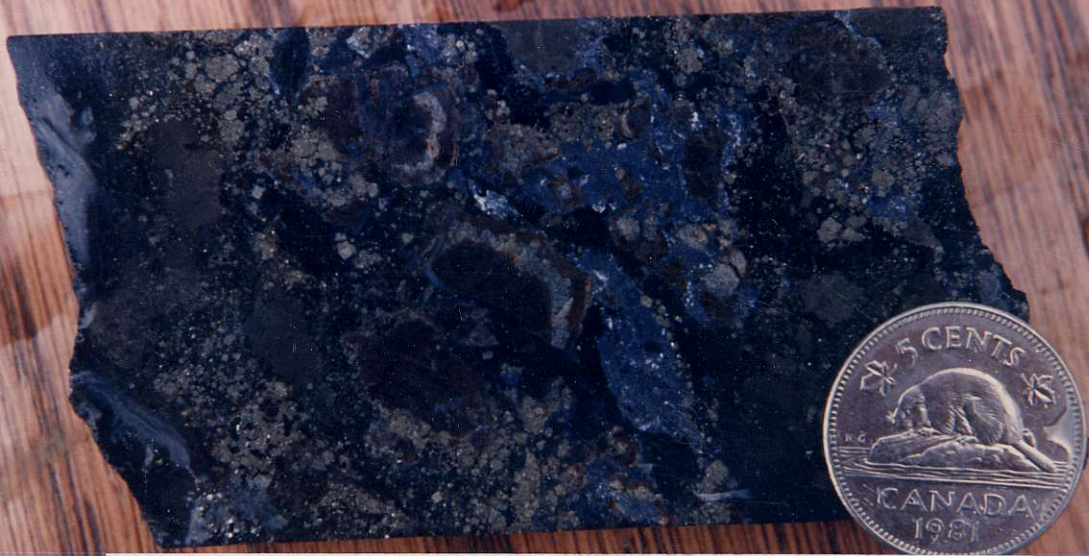
Coarse, zoned sphalerite and galena, Contact Unit, 21B Deposit, Eskay Creek, DDH CA89-109: 90.5m.
