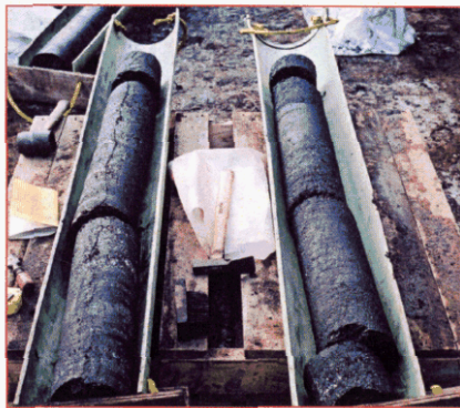
J seam bulk sample core (150 mm), December 2002.
