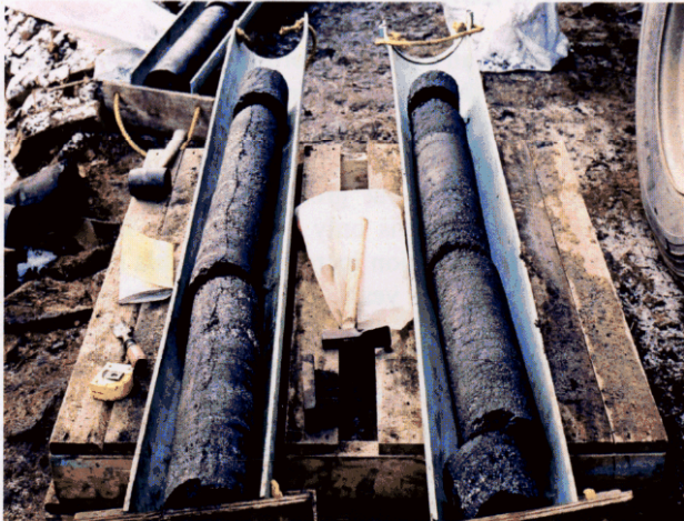
J Seam bulk sample core (150mm) December 2002
