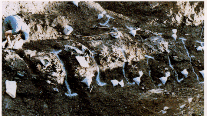
Open cut showing high grade silver-lead-zinc ore in the "C" vein
