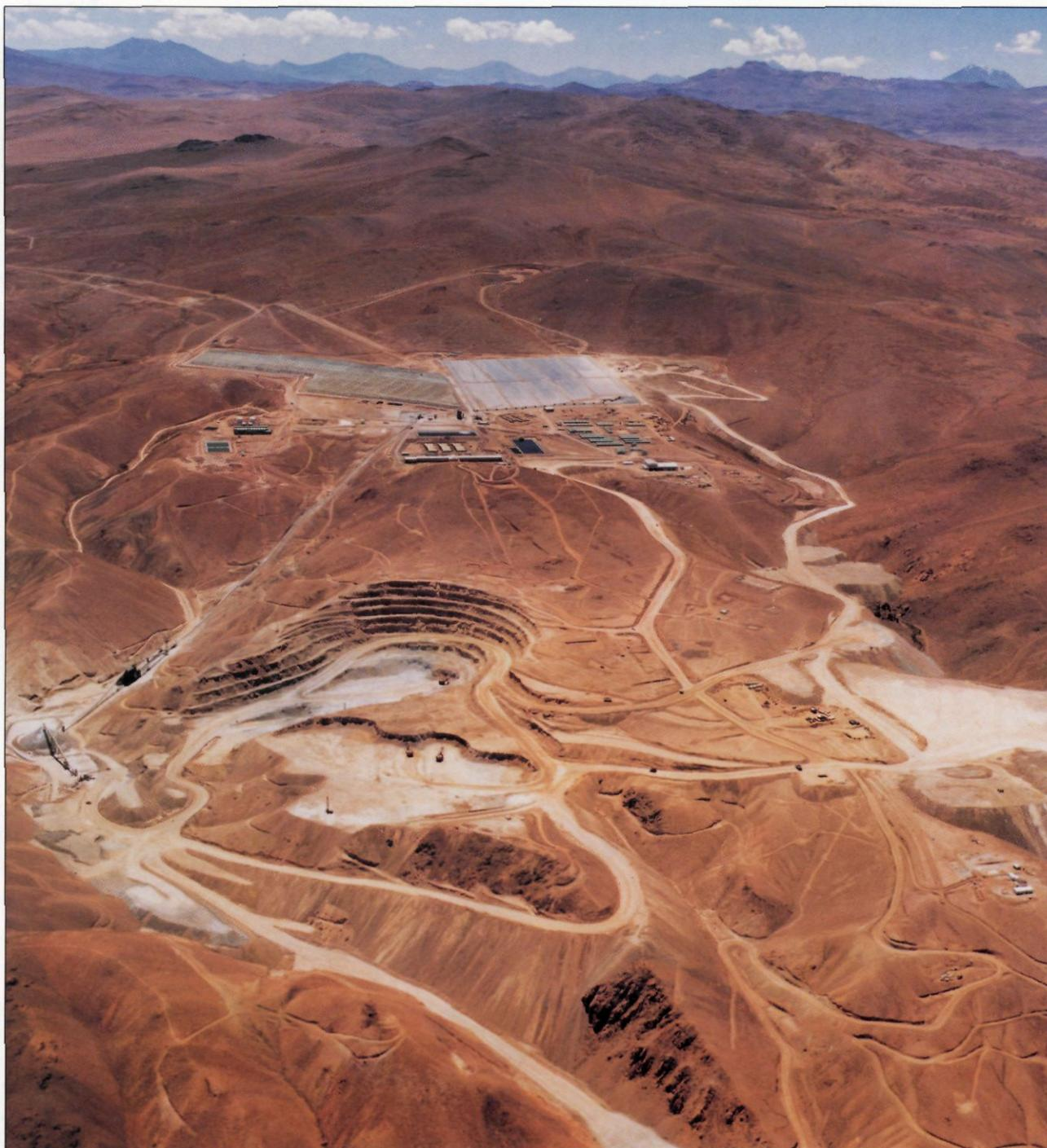
Facing page: An aerial of the facilities show the solvent extraction and electrowinning plants on the left and the offices and accommodations on the right. Inside the electrowinning plant, where cathode copper is produced in seven-day cycles; This page: An overview of the entire operation; ore from the pit is stockpiled and crushed (left) before being transported by conveyors to the agglomerators. The leach pads are at the top.
