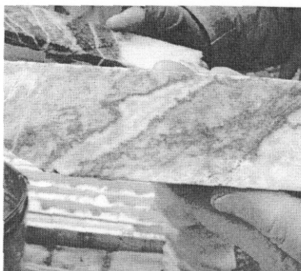
A half-section of diamond drill core from hole TT-16 showing typical high-grade gold-silver mineralization from the Ted Vein. This hole returned 28 metres grading 3.78 grams gold/tonne and 137.5 grams silver/tonne.
