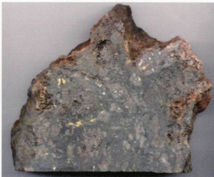
Massive pyrite-enargite-tetrahedrite boulder from Tamdhu showing area - 12.05 % copper, 22.1 g/t gold and 2413 g/t silver
