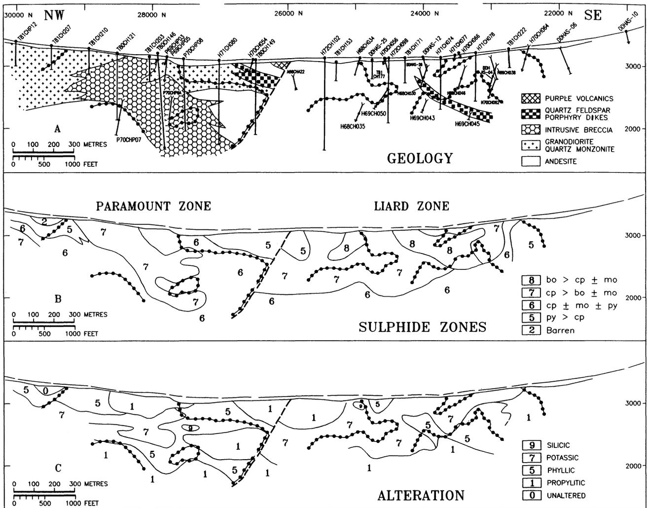
FIGURE 5. Longitudinal section: A — geology; B — sulphide zones; C — alteration facies.
