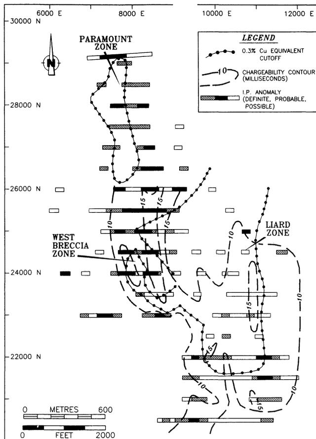
FIGURE 3. Induced polarization surveys.
