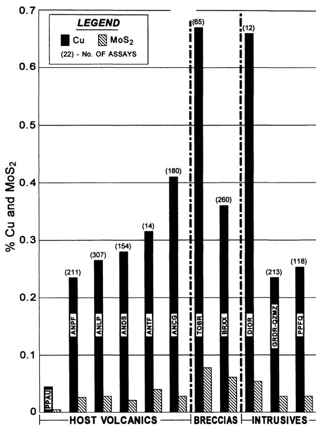
FIGURE 6. Average Cu and MoS<sub>2</sub> content for different rock types (see text for rock codes).
