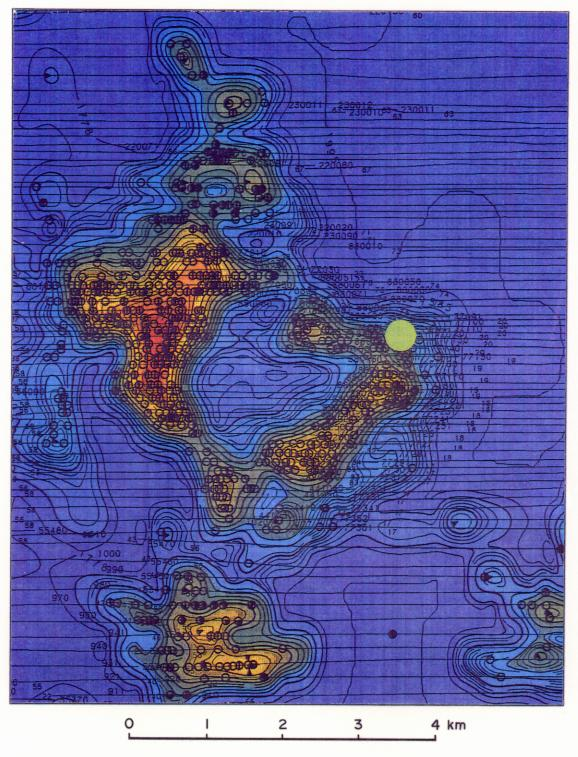
Resistivity anomaly around the Goldslide Intrusion. The Marc Zone location is the large colored dot. The resistivity anomaly follows the hydrothermal alteration.
