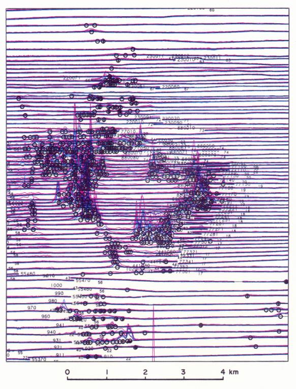
Electromagnetic profiles anomaly around the Goldslide Intrusion. In the Marc Zone area the anomalies are caused by massive sulphide vein and stockwork mineralization in hydrothermal altered vocanic breccias.
