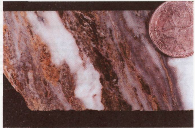
FIGURE 17. Laminated calcite + chlorite + sericite + pyrite + Fe-carbonate vein from drill hole U94-1120, 114 m.
