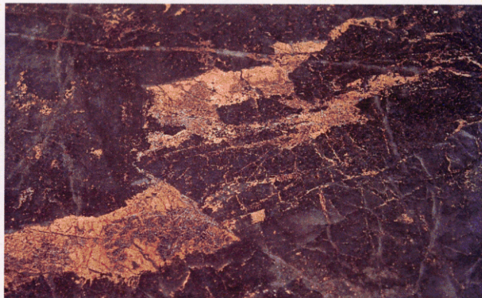
Photograph of a piece of high-grade drill core from the East Zone with significant chalcopyrite, bornite and pyrite minerals present.
