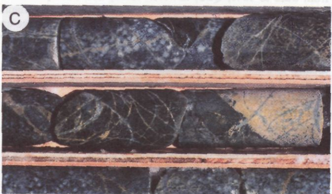
FIGURE 9c. Secondary K-spar along veinlets and fractures within QD2 and QD3 units (K-spar stained yellow by sodium cobaltinitrite).
