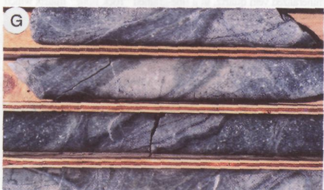
FIGURE 9g. Sharp borders between dark potassium silicate alteration (with abundant hydrothermal biotite) and later, pale sericite-iron carbonate-clay alteration; several borders are coincident with quartz veinlets.
